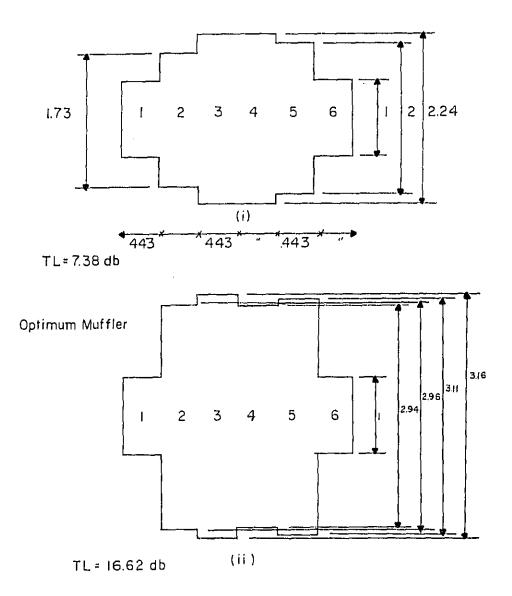
FIG.(5-C) Six Segment Reactive Muffler
