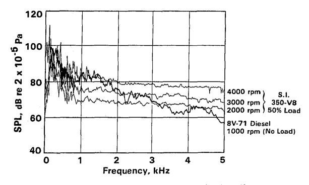
Figure 2. Radiated Exhaust Noise from Two Unsilenced Engines (measured 1.5 m from the end and 45° off the axis of the tailpipe).
