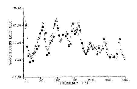
Figure 7. Transmission loss of prototype muffler; +=twomicrophone, random-excitation method; •=standingwave method.
