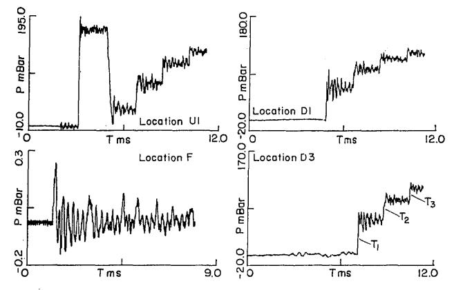
FIGURE IS PRESSURE HISTORIES OF SHOCK PROPAGATION THROUGH EXPANSION CHAMBER, C. Ms = 1.07, SHOCK TUBE
