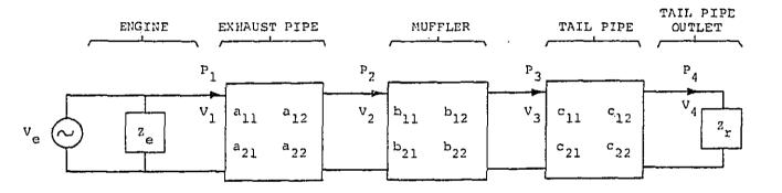
Figure 3. Representation of engine and exhaust system using four-pole theory.
