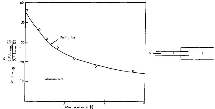
2(b). ACOUSTIC ENERGY TRANSPORT AT AN EXPANSION WITH SIDE BRANCH FIG.
