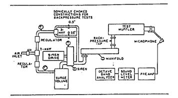
FIGURE 2 Schematic of Bench Test Facility
