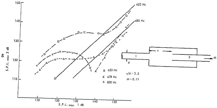
9. FLOW ACOUSTIC COUPLING AT AN AREA EXPANSION. FIG.
