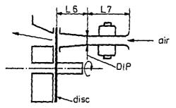
Fig.9 induction tract length/diameter characteristics for disc value engines.
