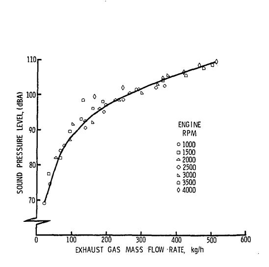
Figure 3. Radiated Exhaust Noise Versus Exhaust Gas Mass Flow Rate for a V-8 Engine.
