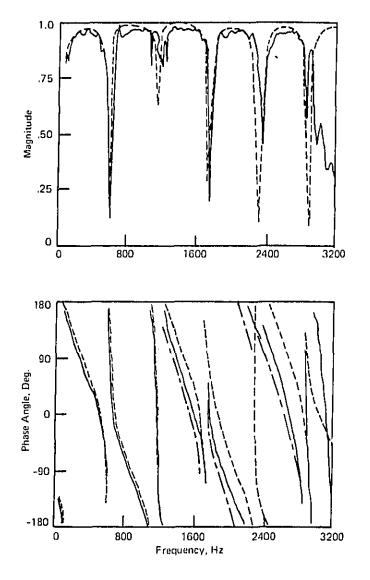
Figure 12. Magnitude and Phase Angle of the Reflection Coefficient for the Expansion Chamber Silencer; --- theory, --- modified theory, --- experiment.
