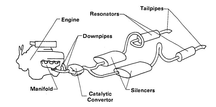
Figure 1. Components of an Engine Dahaust System.
