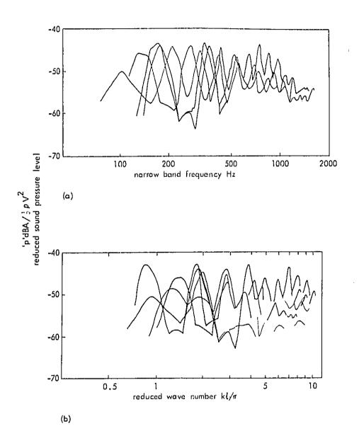
FIG. 14 OPEN PIPE MEASUREMENTS, FULL LOAD. FOUR CYLINDER FOUR CYCLE PETROL ENGINE. 2000 < N < 52:50 rpm
