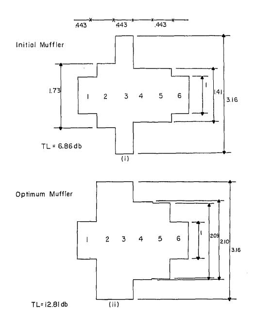
FIG.(5-b)Six Segment Reactive Muffler
