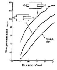
Fig. 8 Effect of the gap of inlet and outlet expansion pipe to flow generated noise
