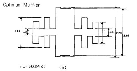
FIG.(6-a) Twelve Segment Reactive Muffler
