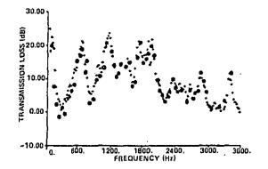
Figure 8. Measured Values of Transmission Loss for Prototype Automotive Muffler. Filled Circle: SWR Method; Open Square, Plus Sign: Two-Microphone Random-Excitation Method
