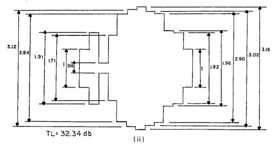
FIG.(6-b) Twelve Segment Reactive Muffler
