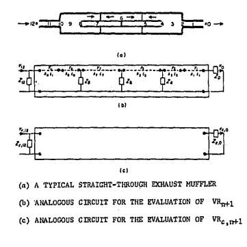
Figure 1. FORMULATION FOR VELOCITY RATIO-CUM-TRANSFER MATRIX METHOD.
