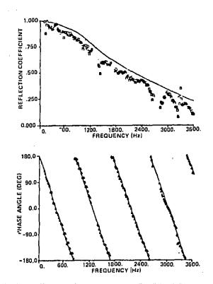
Figure 7. Power Reflection Coefficient and Phase Angle for Open End Tube. Solid Line: Theory; Open Square, Open Triangle: experiment.
