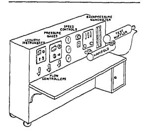
FIGURE 9 Final Prototype Muffler Bench Test Facility
