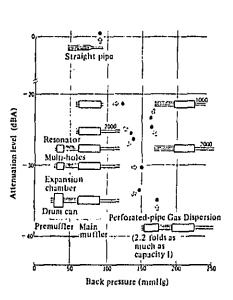
Fig. 22 Relation of exhaust noise reduction and back pressure of various exhaust system arrangements
