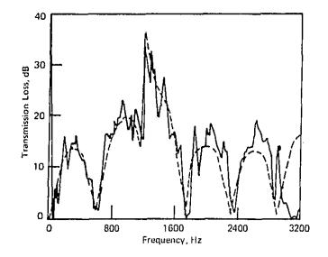
Figure 13. Transmission Loss for the Expansion Chamber Silencer; --- theory, --- experiment.
