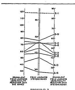
FIGURE 7 Comparison of Field and Facility Evaluations of Muffler Performance
