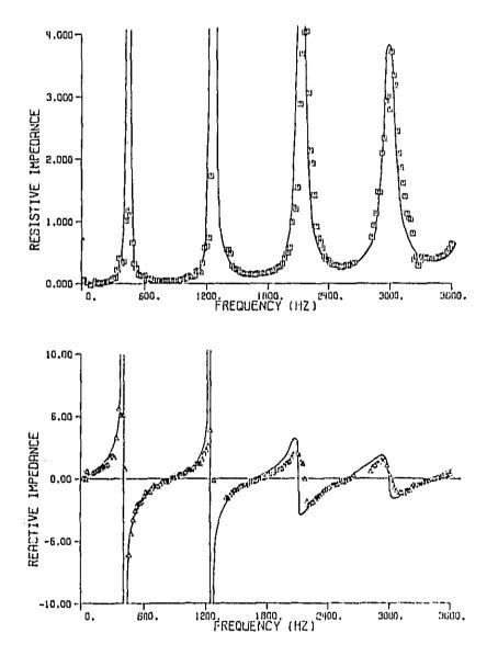
Figure 6. Resistive and reactive tail pipe impedances; solid line=theory; symbols=experiment.
