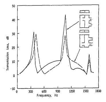
Figure 24. Predicted Transmission Losses for Combination of SI-CO Flow-Reversing Chamber and Helmholtz Resonator, With Different Throat Locations: ---- Side-Located Throat and ------ Centrally Located Throat
