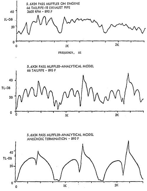
Figure 15. Analytical and Experimental Results for a Pass Muffler.
