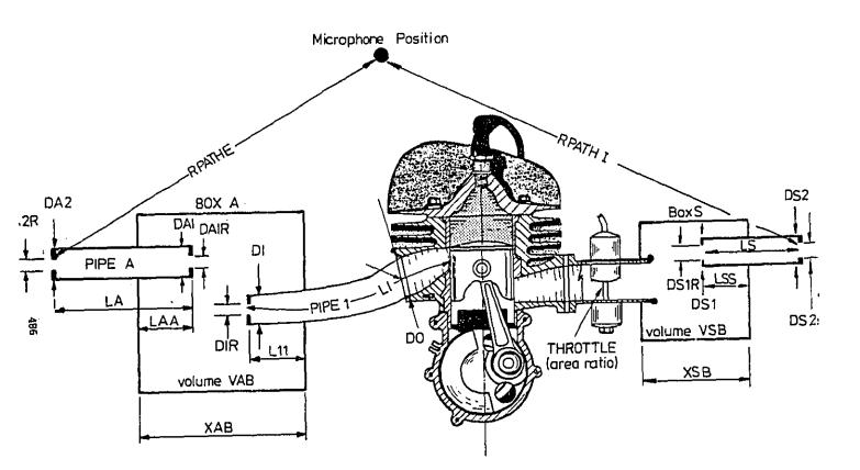
Program: G.P.B.1 EXHAUST AND INTAKE SILENCING BOX PARAMETERS REQUIRED FOR PROGRAM
