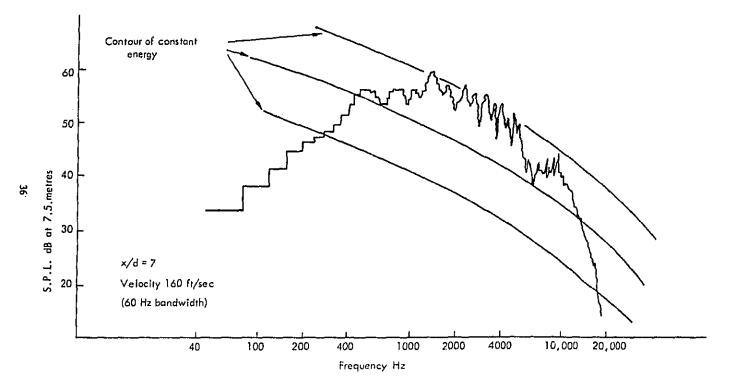
FIG. 5. SPECTRAL CONTENT OF FLOW NOISE
