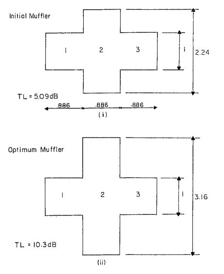
FIG.(4) Three Segment Reactive Muffler
