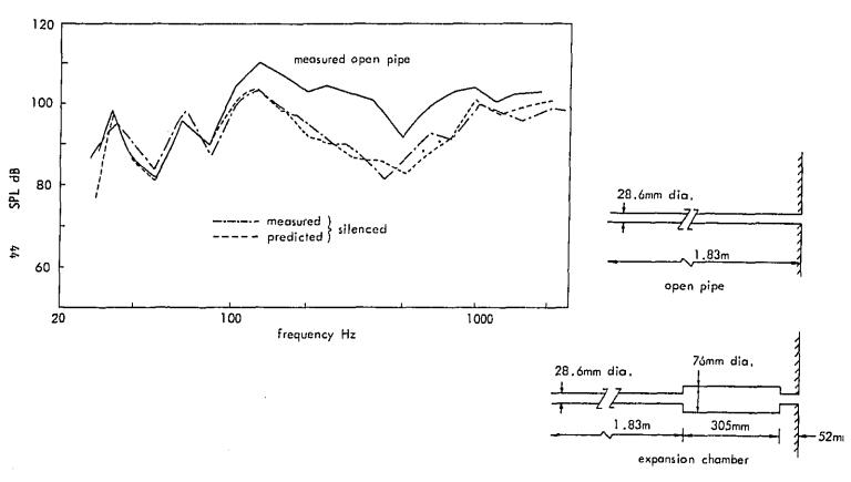
FIG. 13 SINGLE EXPANSION CHAMBER PERFORMANCE CONSTANT VOLUME VELOCITY SOURCE LINEAR ACOUSTIC ANALYSIS
