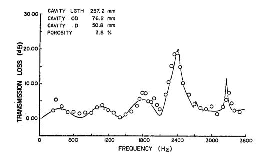
Figure 29. Transmission Loss for a Long Resonator, (Predicted ------ Measured o)
