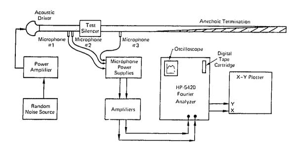
Figure 9. Test Arrangement and Instrumentation.
