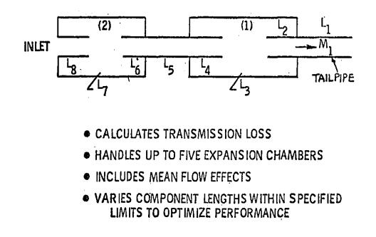
Figure 5. FEATURES OF NASA MUFFLER DESIGN COMPUTER PROGRAM.
