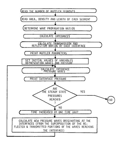
Fig. 2 Block diagram of analysis program
