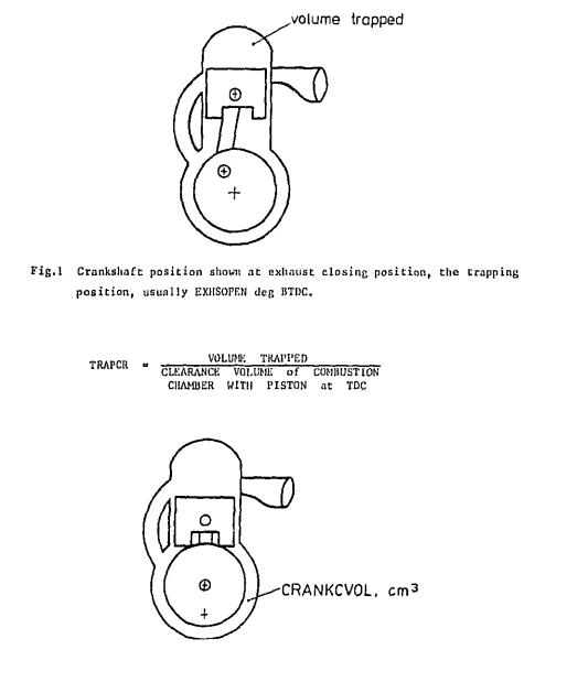
Fig.2 Crankshaft position shown at bottom dead centre, B.D.C. - note all transfer ducts are open, and the volume under the piston is then the crankcase clearance volume, measured in  $Cm^3$ . If SV is the swept volume per cylinder,  $Cm^3$  then -
