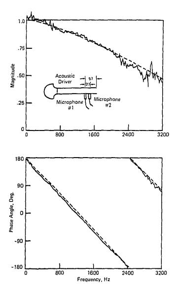
Figure 10. Magnitude and Phase Angle of the Reflection Coefficient for an Open Pipe Termination; --- theory, --- experiment, (dimensions in mm).
