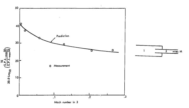
FIG. 1(b) ACOUSTIC ENERGY TRANSPORT AT A CONTRACTION WITH SIDEBRANCH.
