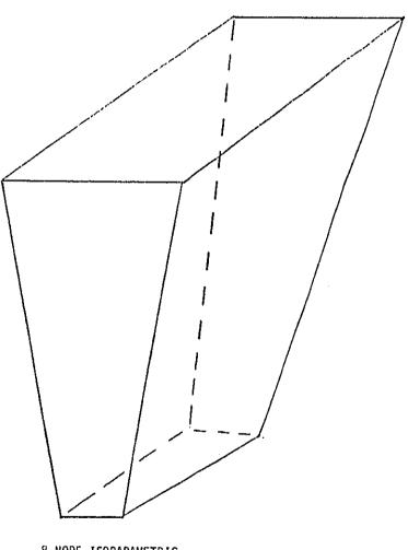
8 NODE ISOPARAMETRIC ACOUSTIC ELEMENT
