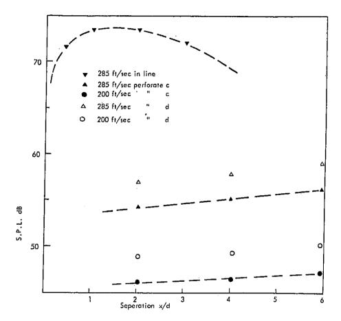
FIG. 7. FLOW NOISE REDUCTION BY PERFORATES.
