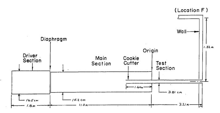
FIGURE 4 GALCIT SIX INCH SHOCK TUBE
