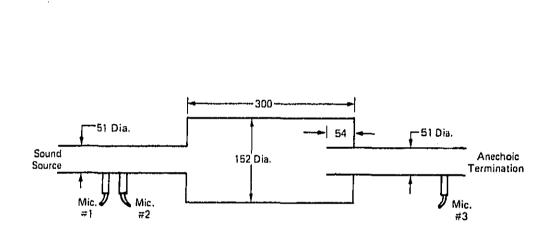
Figure 11. Expansion Chamber Silencer (dimensions in nm).
