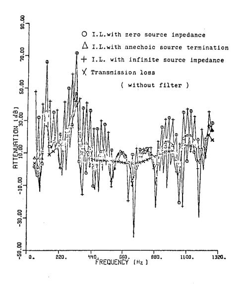
Figure 31. Theoretical Insertion Losses and Transmission Loss for Engine Exhaust Muffler System with Actuat Exhaust Temperature Profile at Firing Frequency 100 Hz
