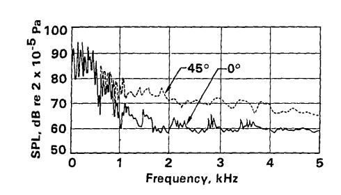
Figure 6. Exhaust Noise Spectra at 0° and 45° from the Tailpipe Axis and 1.5 m from the End of the Tailpipe.
