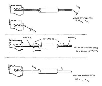
Figure 4. Definitions of Muffler Performance
