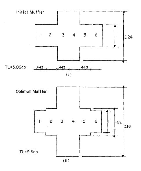
FIG.(5-a) Six Segment Reactive Muffler
