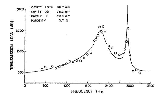
Figure 28. Transmission Loss for a Short Resonator, (Predicted -----, Measured o)
