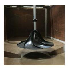
enhances agglomeration of the flakes and avoids loading the flakes. The bigger and more stable these flakes are, the more easily they can be separated in the subsequent purification steps.
