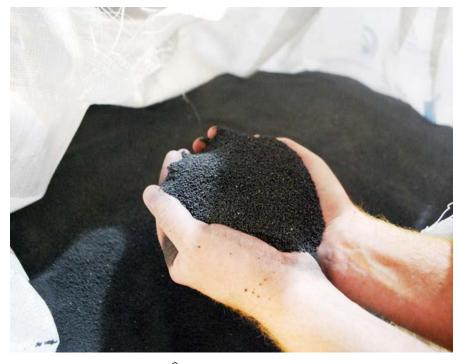
With its large surface area, Filtralite<sup>®</sup>, an expanded clay media, provides an optimal environment for naturally occurring bacteria that oxidize contaminants during filtration.
