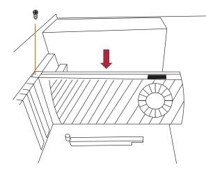
5. Graphics cards in NA265A-G4 are provided with supplementary 12+4-pin (16-pin) 12VHPWR power cables from Netstor unit's PSU for sufficient power. Up to four graphics cards are allowed to be installed in slots 2 ~ 5 within the Netstor chassis.
