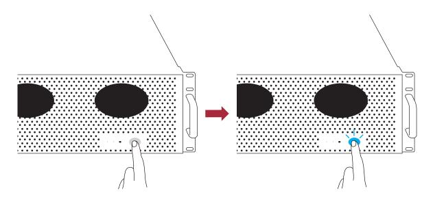
2. To disconnect NA265A-G4 from server, always power off server first, and then power off NA265A-G4. To power off NA265A-G4, press and hold the power LED button for over two seconds until LED button's blue light goes off.
