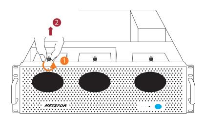
2. The front 9×9 cm cooling fan speed can be adjusted. Pull out the fan module; there will be four sets of pins marked with 6V, 8V, 10V, and 12V from top to bottom on the fan connector board. The default setting is the jumper being placed over pin 5 and pin 6 for 8V as the most-balanced medium speed. Additionally, according to the application situation, user can set it to 10V for higher speed / 12V for highest speed, or set it to 8V for lowest speed.
