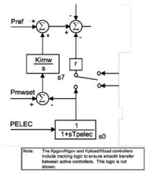
Figure 1.3: GGOV1 Natural Gas Turbine-Governor Model [Source: PSS®E]
