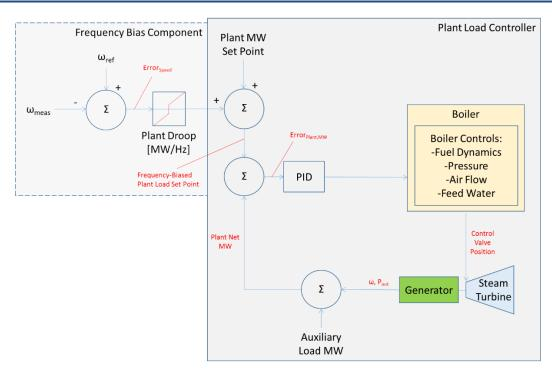
Figure 1.8: Simplified Control Diagram of a Load Controller with Frequency Bias [Source: Adapted from GE]
