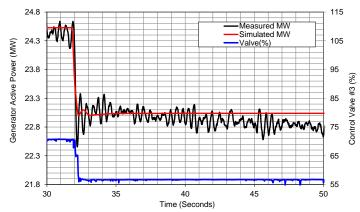
Figure 1.6: Governor frequency step response test with load controller disabled (IEEEG1)
