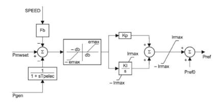
Figure 1.5: LCFB1 Load Controller Model [Source: PSS®E]
