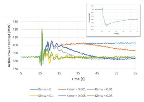
Figure 1.4: Impact of Kimw on Return to MW Set Point in GGOV1
