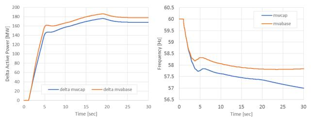
Figure 1.12: Illustration of Response using Machine Base versus Turbine Rating [Source: GE]
