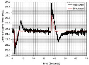
Figure 1.7: (b) Governor frequency step response test with load controller enabled (IEEEG1 + LCFB1)
