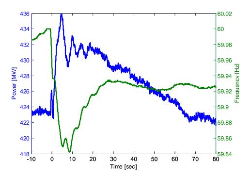
Figure BG.4: Nonsustained Frequency Response–Load Control [Source: BPA]
