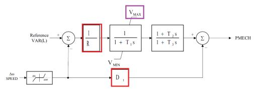
Figure 1.10: Annotated TGOV1DU Model for Conversion from TGOV1 [Source: Adapted from PSS®E]
