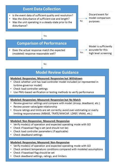
Figure 2.1: Overall Process for Analyzing Expected versus Actual Response
