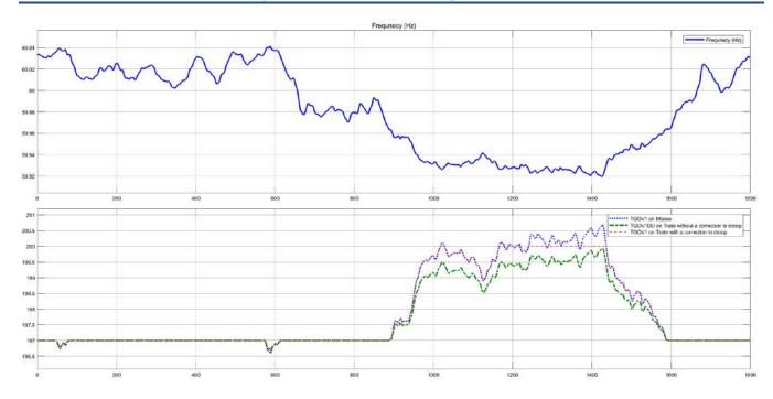
Figure 1.11: Illustration of Response in Converting from TGOV1 to TGOV1DU Model
