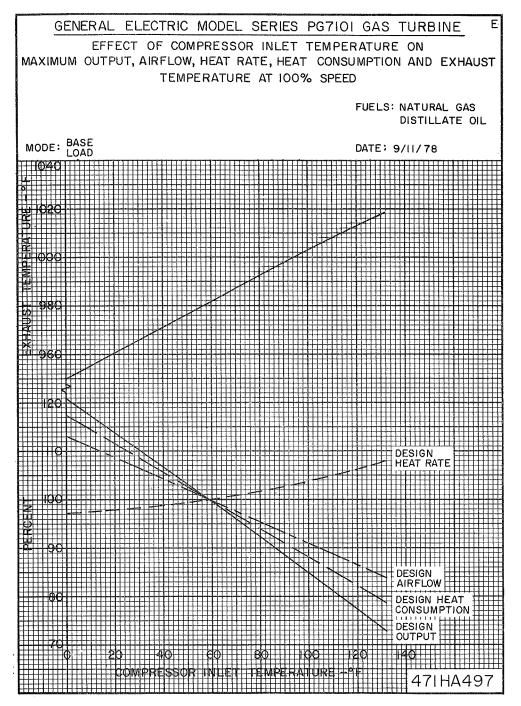
Figure C.2: Inlet Temperature versus Output Curve [Source: GE]
