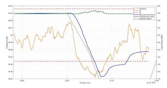
Figure D.5: Inconclusive SCADA Data Due to Machine Ramping to Different Set Points during Frequency Event
