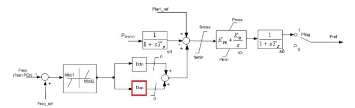
Figure E.1: Plant-Level Controller – Active Power Controls [Source: PSS<sup>®</sup>E]
