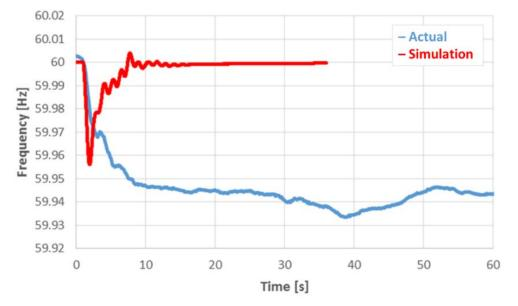
Figure I.1: Simulated vs. Actual Frequency for Large Disturbance
