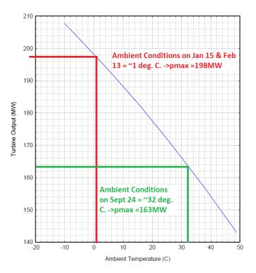
Figure D.4: Power-Ambient Temperature Curve [Source: IESO]
