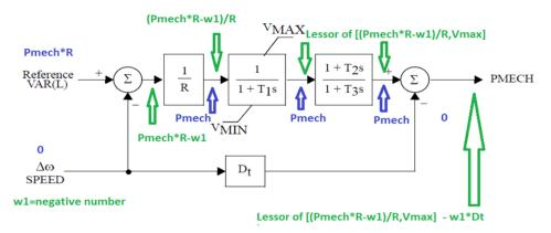
Figure B.1: Annotated TGOV1 Block Diagram
