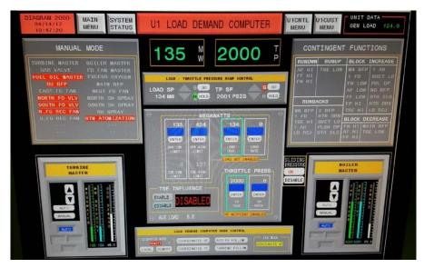
Figure 1.9: Steam Turbine Load Demand Controller [Source: Entergy]
