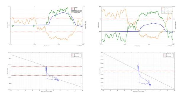
Figure D.1: Measured vs. Actual Performance – Match with Proper Intentional Deadband (Left), Overestimated Performance with Improper Deadband (Right)
