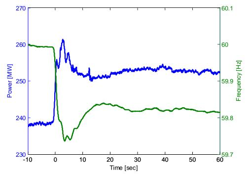
Figure BG.3: Sustained Primary Frequency Response [Source: BPA]
