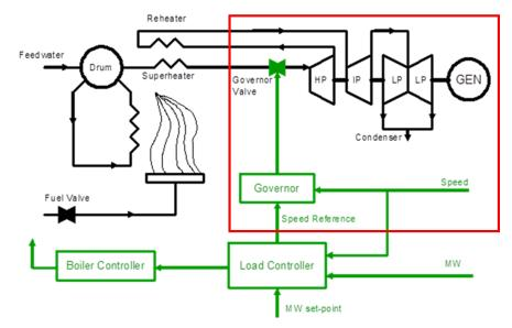
Figure BG.2: High Level Block Diagram of Related Turbine-Governor Controls [Source: BPA]
