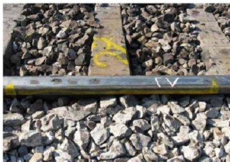
Figure 6. Lamination in rail in 49 mm depth with 300 mm length
