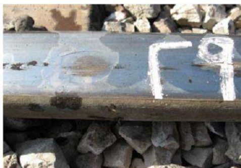
Figure 6. Lamination in rail in 49 mm depth with 300 mm length
