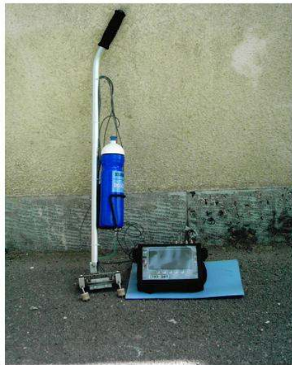
Figure 1. Walking stick ultrasonic testing device
