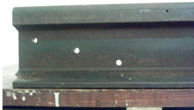
Figure 2. The calibration block with defined defects
