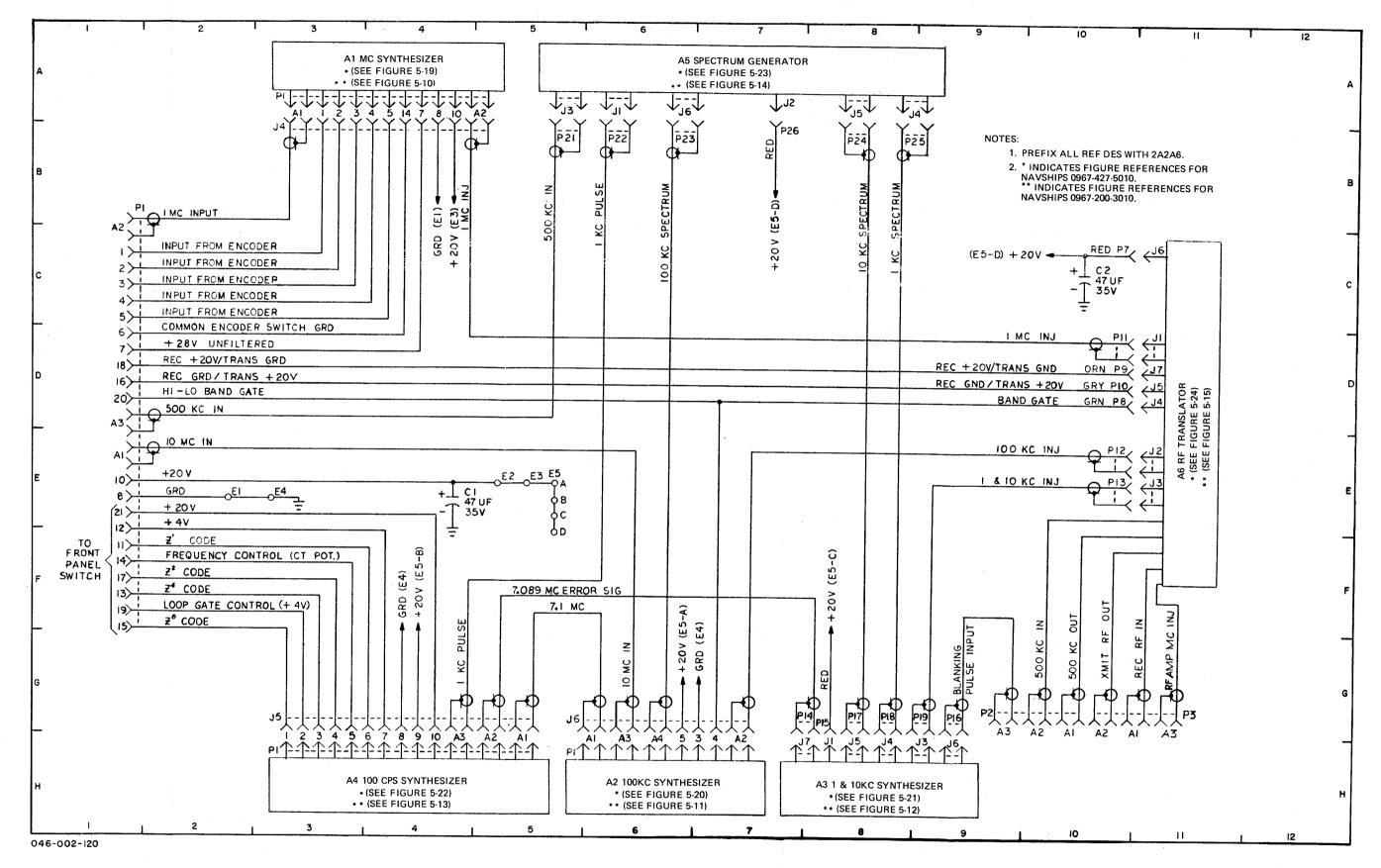
Figure 5-18. Translator/Synthesizer Assembly 2A2A6, Schematic Diagram
