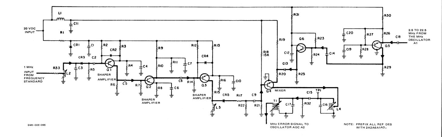
Figure 3-43. T-827B/URT, Spectrum Generator/Mixer, Simplified Schematic Diagram
