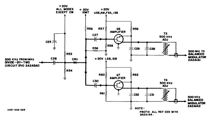
Figure 3-13. T-827B/URT, 500-kHz Amplifiers, Simplified Schematic Diagram
