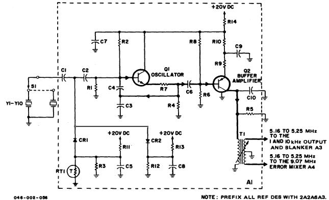
Figure 3-38. T-827B/URT, 5.16- to 5.25-MHz Oscillator, Simplified Schematic Diagram
