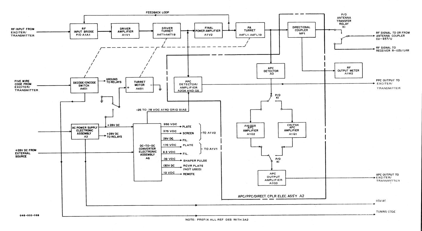
Figure 3-52. Radio Frequency Amplifier AM-3007/URT, Functional Block Diagram
