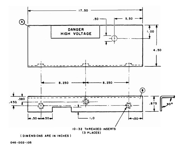
Figure 5-3. Special Capacitance Shield for AM-3007/URT
