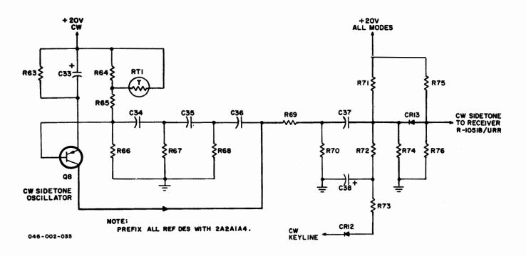
Figure 3-20. T-827B/URT, CW Sidetone Oscillator/Gate, Simplified Schematic Diagram
