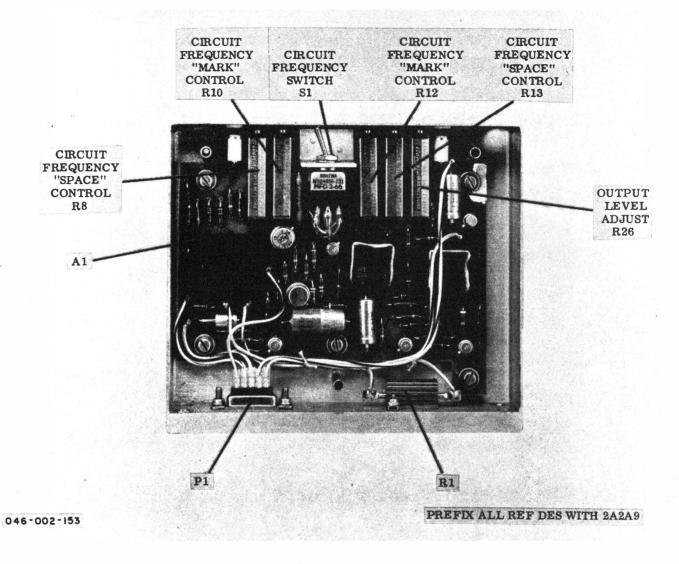
Figure 5-51. FSK Tone Generator Assembly 2A2A9, Component Location
