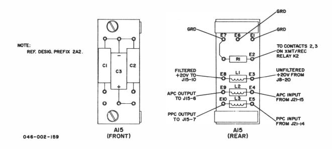
Figure 5-57. Transmitter IF. Filter Assembly 2A2A15, Component Location
