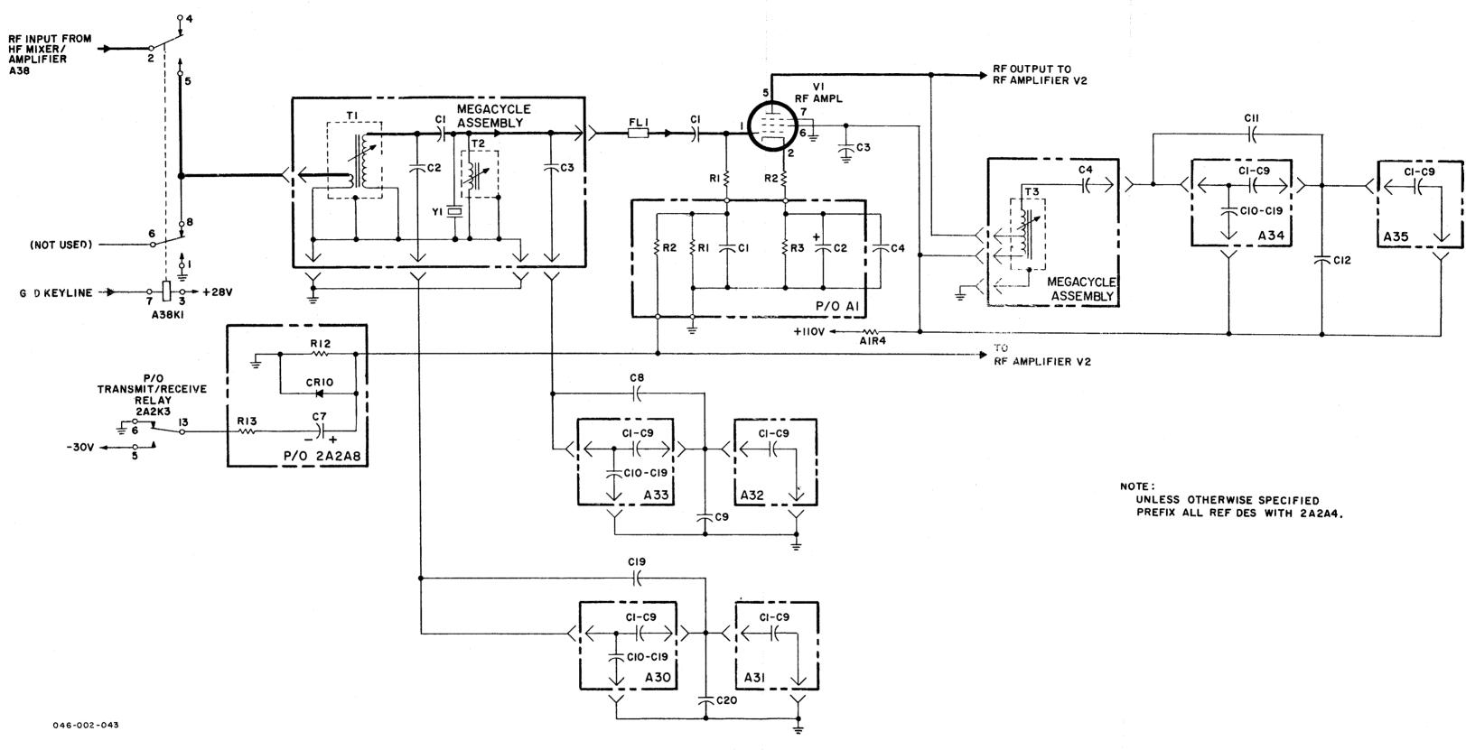
Figure 3-26. T-827B/URT, RF Amplifier V1, Simplified Schematic Diagram
