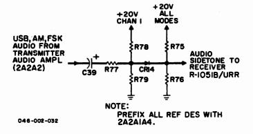
Figure 3-19. T-827B/URT, Sidetone Gate, Simplified Schematic Diagram
