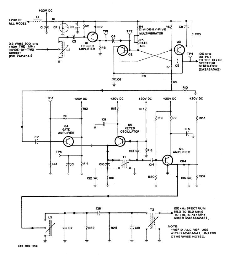
Figure 3-34. T-827B/URT, 100-kHz Spectrum Generator, Simplified Schematic Diagram
