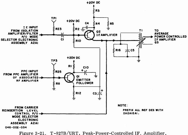
gure 3-21. 1-827B/URT, Peak-Power-Controlled IF. Amplific Simplified Schematic Diagram
