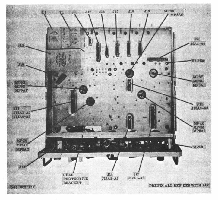
Figure 5-35. T-827B/URT Chassis Less Assemblies, Top View, Component Location
