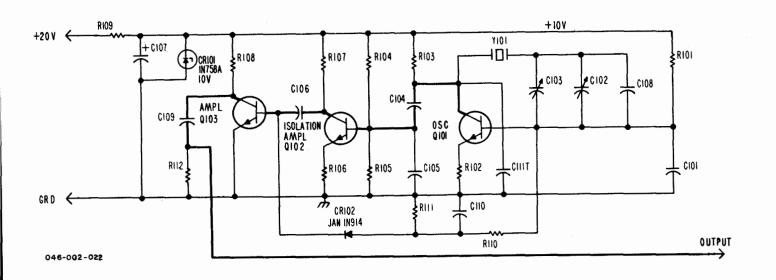
Figure 3-9. T-827B/URT, Typical 5-MHz Oscillator, Simplified Schematic Diagram
