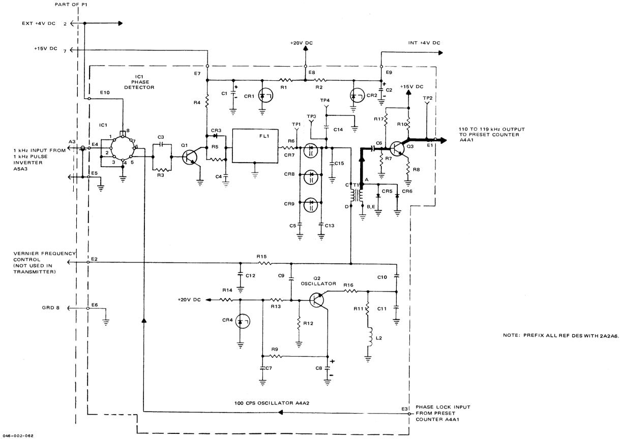
Figure 3-46. T-827B/URT, 100-Hz Oscillator, Simplified Schematic Diagram
