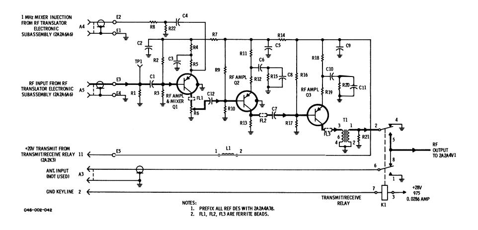
Figure 3-25. T-827B/URT, Mixer/Amplifier, Simplified Schematic Diagram NAVSHIPS 0967-427-5010
