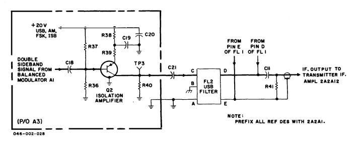
Figure 3-15. T-827B/URT, Isolation Amplifier/Filter, Simplified Schematic Diagram
