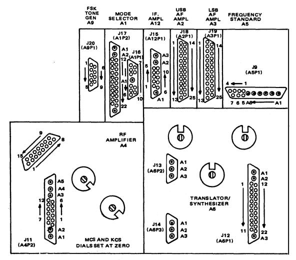
FRONT OF T-8278/URT' ELECTRONIC ASSEMBLIES REMOVED
