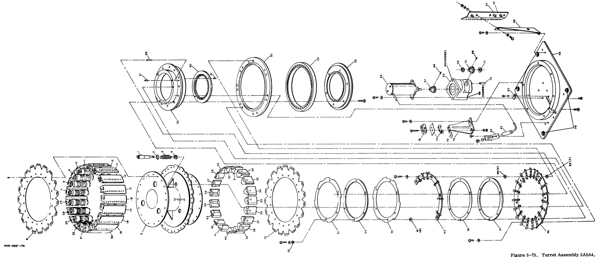
Figure 5-73. Turret Assembly 3A2A4, Exploded View
