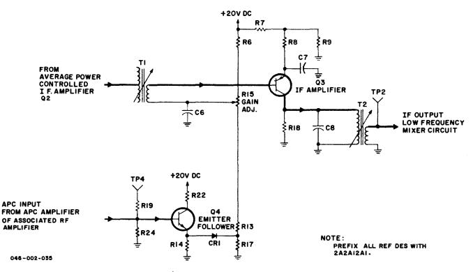
Figure 3-22. T-827B/URT, Average-Power-Controlled IF. Amplifier, Simplified Schematic Diagram
