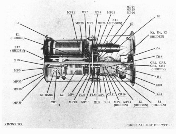
Figure 5-85. Antenna Coupler CU-937/UR Right Side, Component Location
