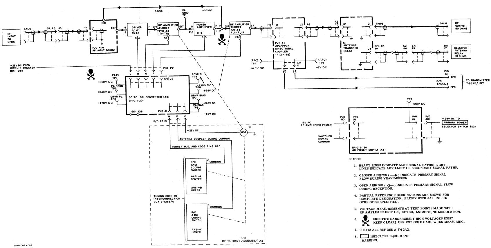
Figure 4-17. RF Amplifier AM-3007/URT, Overall Servicing Block Diagram
