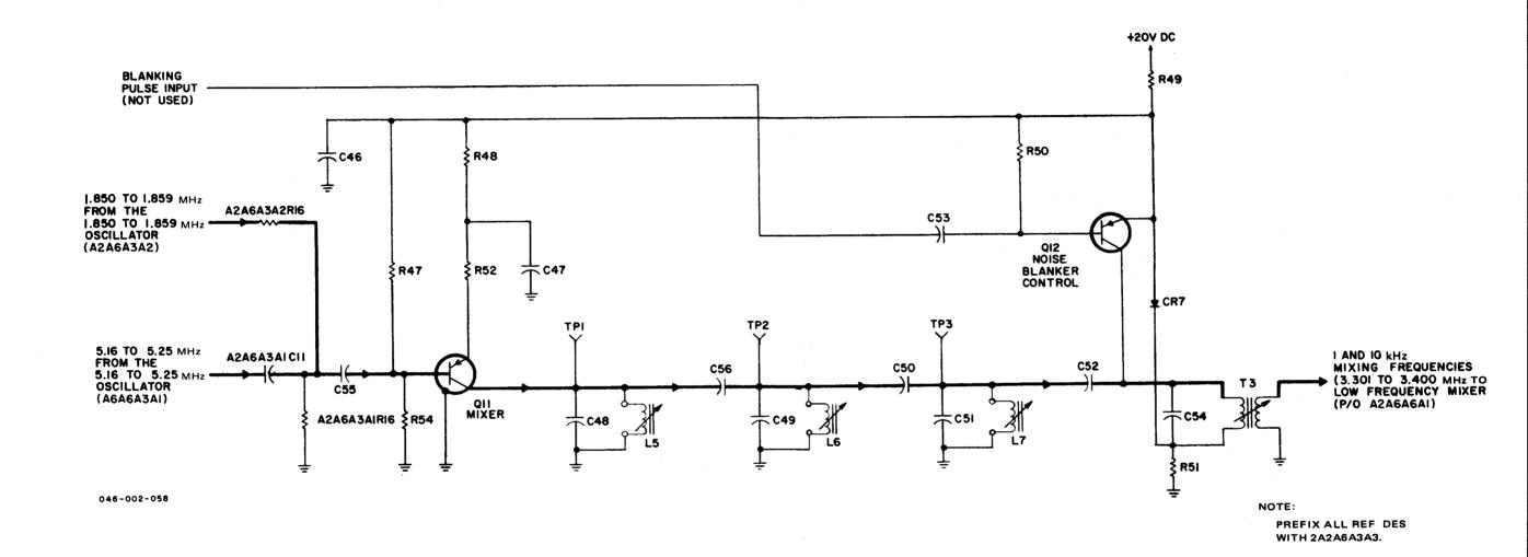
Figure 3-40. T-827B/URT, 1- and 10-kHz Output and Blanker, Simplified Schematic Diagram
