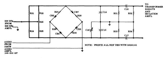
Figure 3-14. T-827B/URT, Balanced Modulator, Simplified Schematic Diagram
