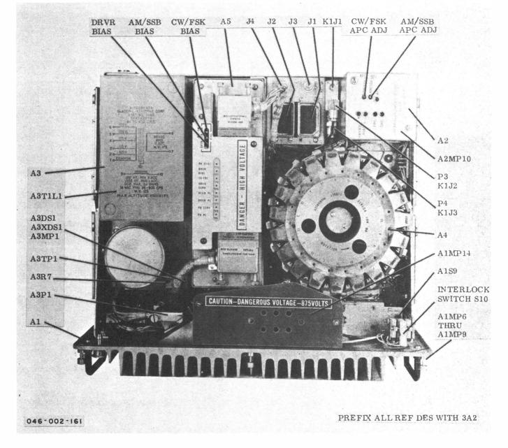
Figure 5-59. AM-3007/URT Chassis, Top View, Component Location
