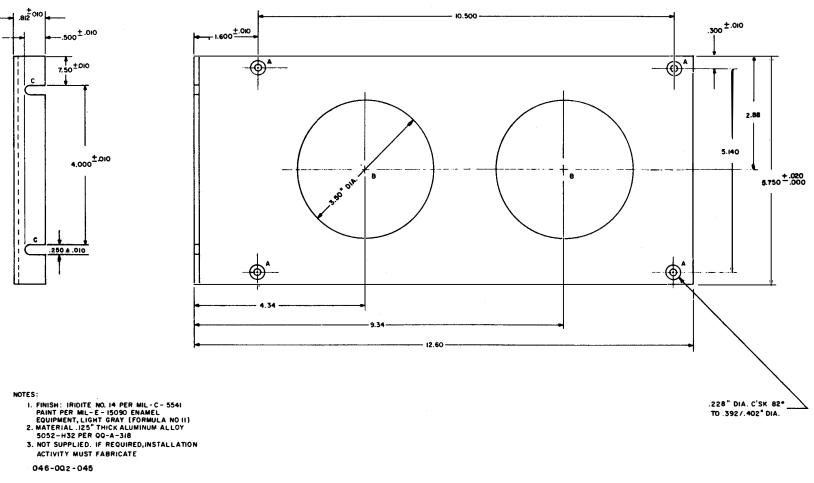
Figure 7-4. Radio Set AN/WRC-1B, Mounting Bracket for Rack Mounting
