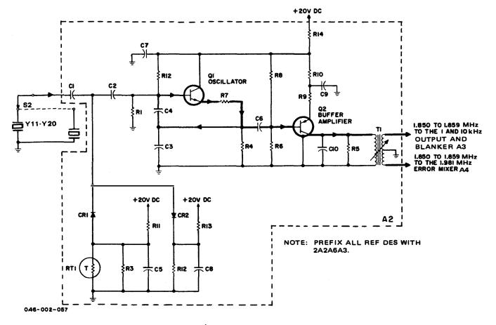
Figure 3-39. T-827B/URT, 1.850- to 1.859-MHz Oscillator, Simplified Schematic Diagram
