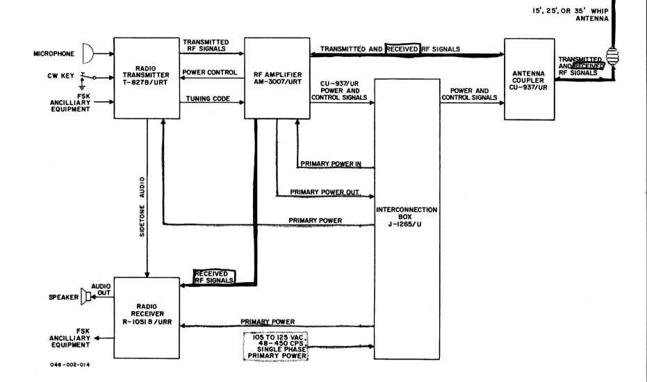
Figure 3-1. Radio Set AN/WRC-1B, Functional Block Diagram
