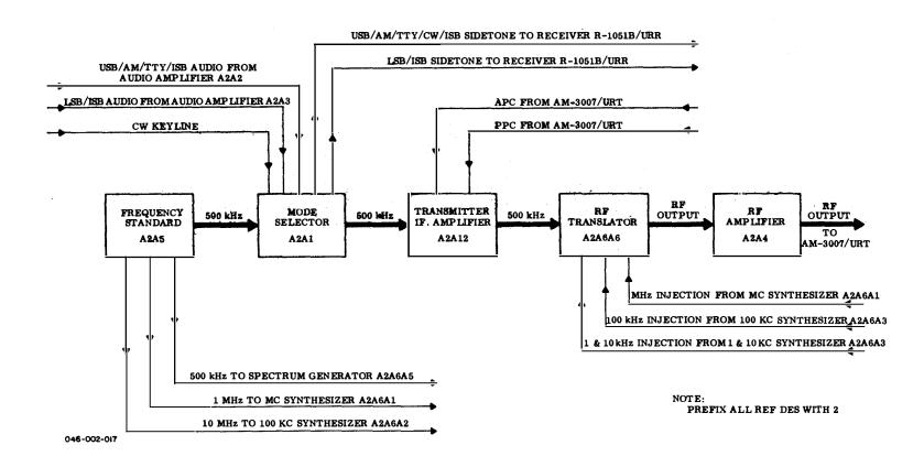
Figure 3-4. T-827B/URT, Main Signal Flow Section, Functional Block Diagram
