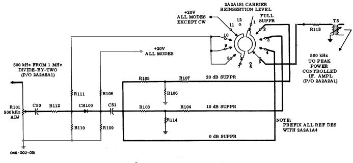
Figure 3-18. T-827B/URT, SSB Carrier Reinsertion Level Control, Simplified Schematic Diagram
