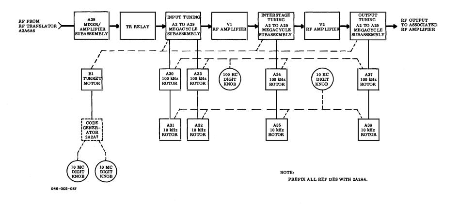
Figure 3-24. T-827B/URT, RF Amplifier, Simplified Block Diagram
