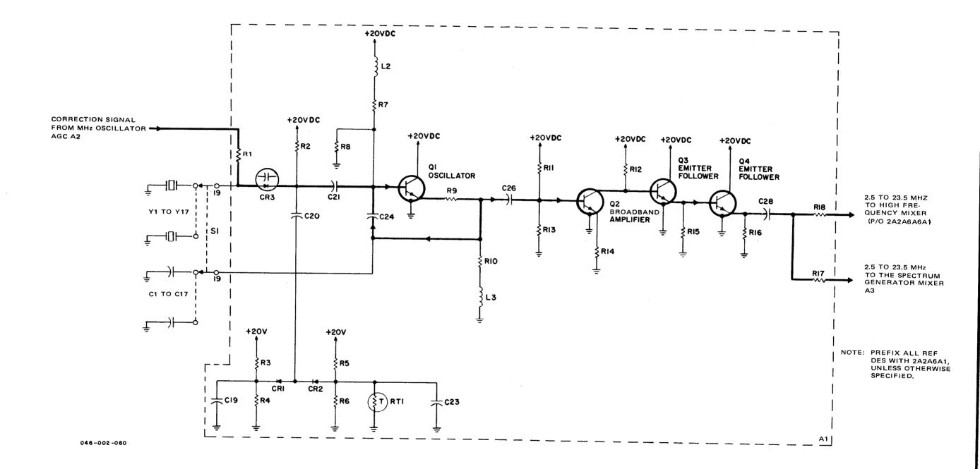
Figure 3-42. T-827B/URT, MHz Oscillator, Simplified Schematic Diagram
