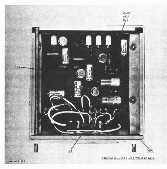
Figure 5-54. Transmitter IF. Amplifier Assembly 2A2A12, Component Location
