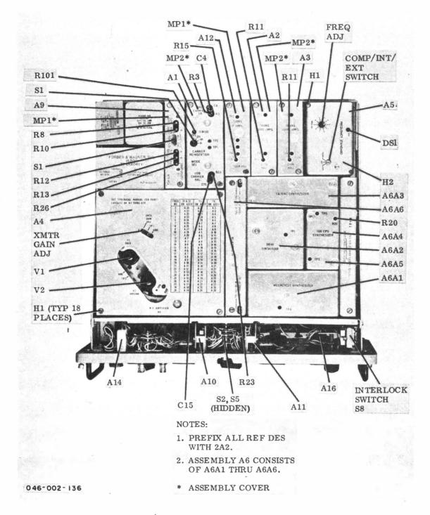
Figure 5-34. T-827B/URT Chassis, Top View, Component Location
