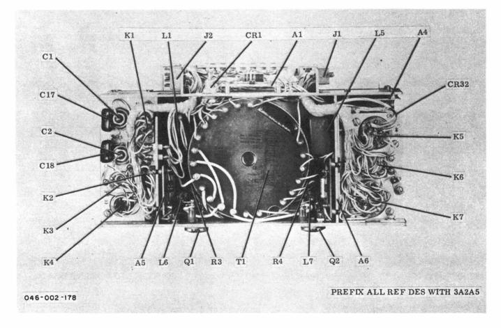
Figure 5-76. DC-to-DC Converter Assembly 3A2A5 Right View, Component Location
