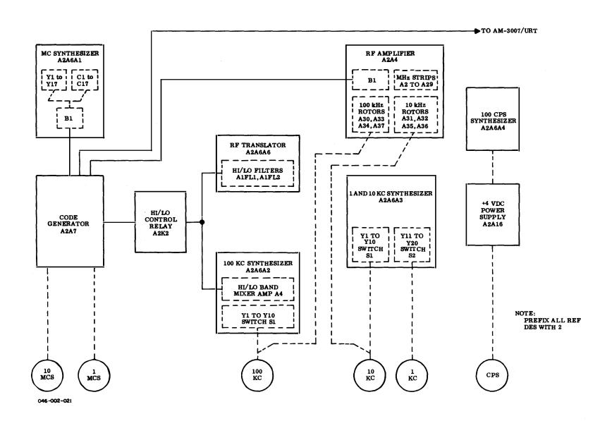
Figure 3-8. T-827B/URT, Digital Tuning, Simplified Block Diagram
