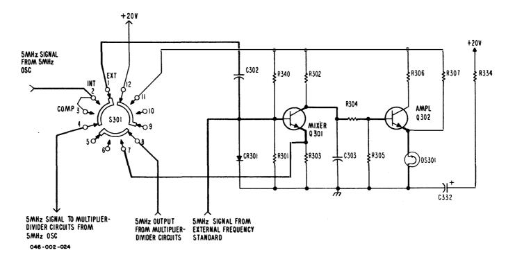
Figure 3-11. T-827B/URT, Typical Comparator, Simplified Schematic Diagram
