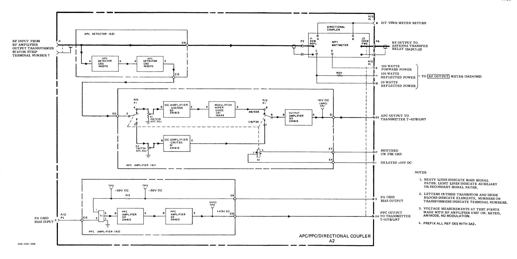
Figure 4-18. APC/PPC/Directional Coupler Assembly 3A2A2, Servicing Block Diagram
