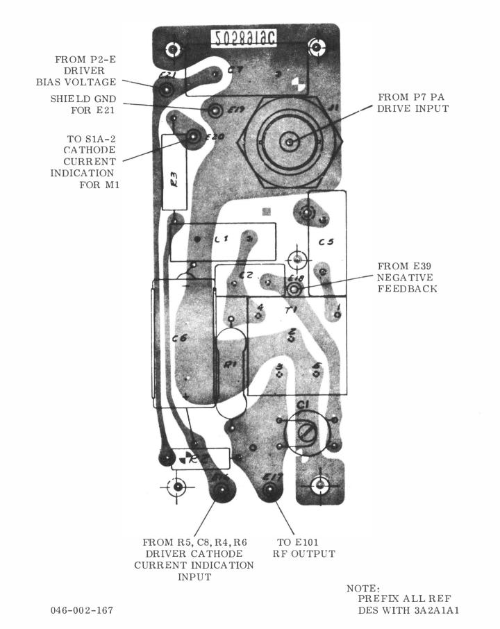
Figure 5-65. RF Input Bridge PCB (3A2A1A1), Component Location
