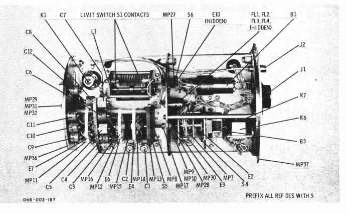
Figure 5-86. Antenna Coupler CU-937/UR Left Side, Component Location
