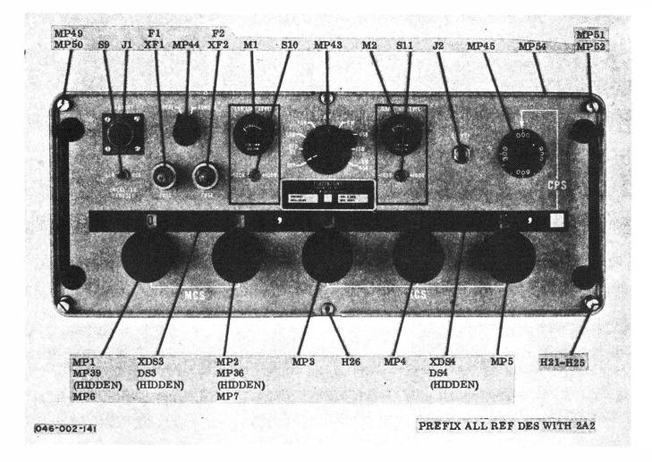
Figure 5-39. T-827B/URT Front Panel, Component Location
