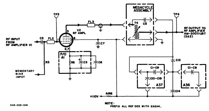
Figure 3-27. T-827B/URT, RF Amplifier V2, Simplified Schematic Diagram
