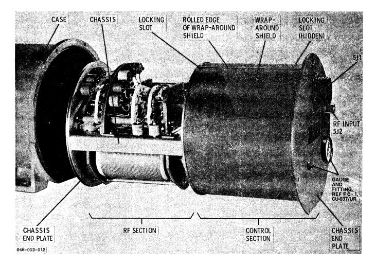
Figure 1-9. Antenna Coupler CU-937/UR, Side View, Case Removed
