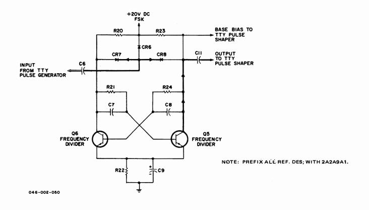
Figure 3-32. T-827B/URT, TTY Frequency Divider, Simplified Schematic Diagram
