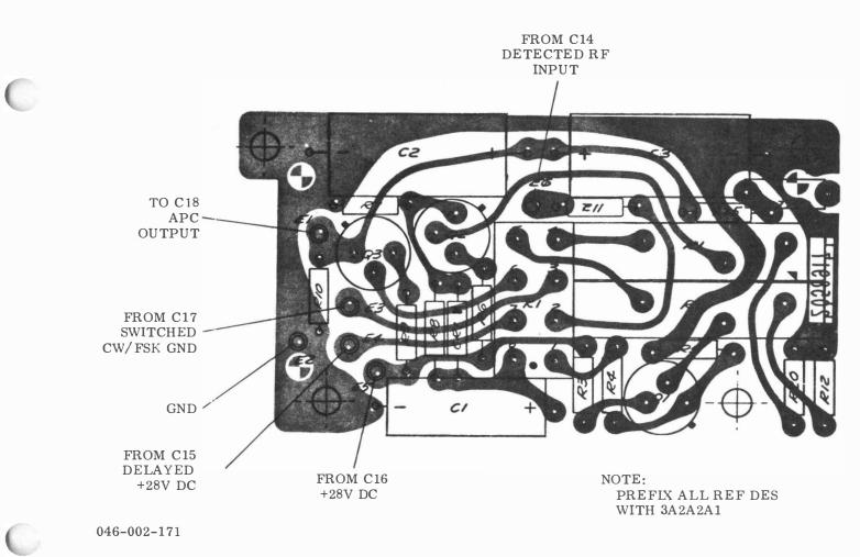
Figure 5-69. APC Amplifier PCB (3A2A2A1), Component Location
