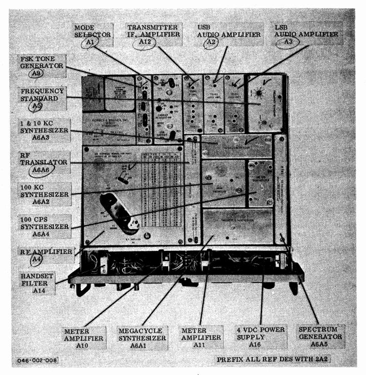
Figure 1-5. Radio Transmitter T-827B/URT, Top View, Case Removed
