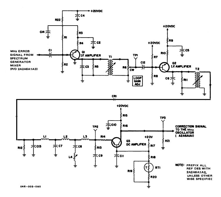
Figure 3-44. T-827B/URT, MHz Oscillator AGC, Simplified Schematic Diagram
