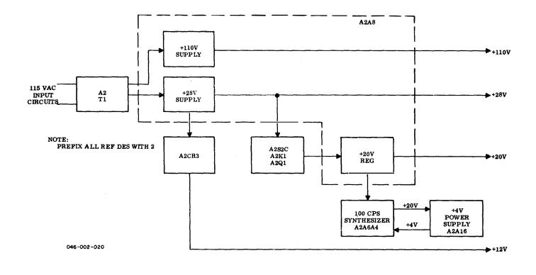
Figure 3-7. T-827/URT, DC Power Supply, Simplified Block Diagram
