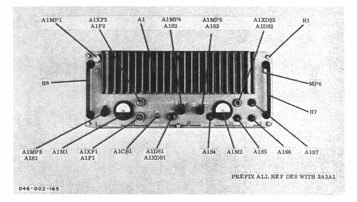
Figure 5-63. AM-3007/URT Front Panel, Component Location
