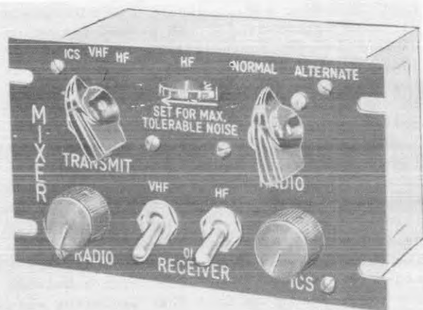
C-242/AIC-4 Pilot's Control Unit Shown Without Blanking Plate Over the ICS Position of the TRANSMIT Switch
