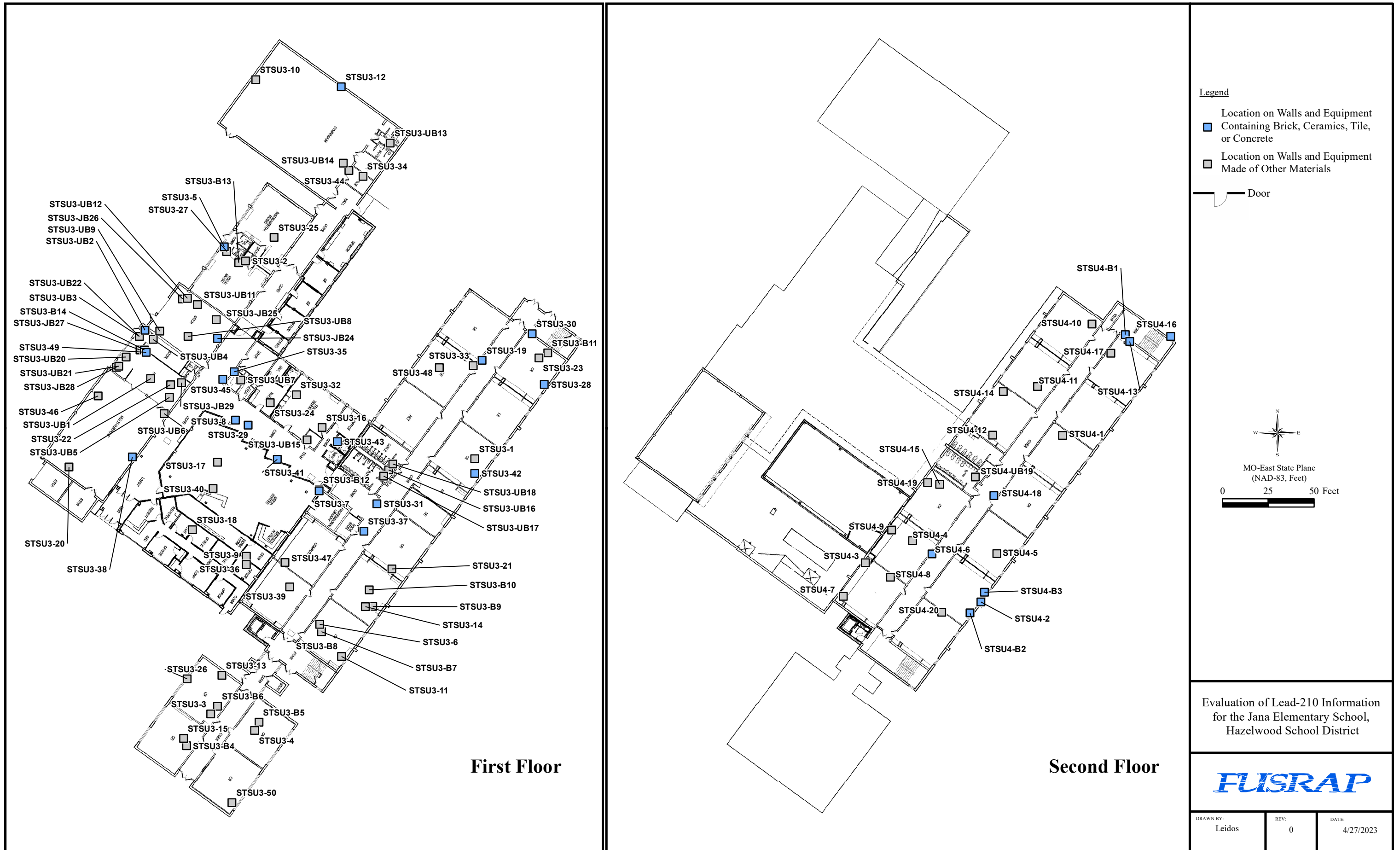
Figure 3. Structure Surface Survey Locations for Interior Walls and Equipment
