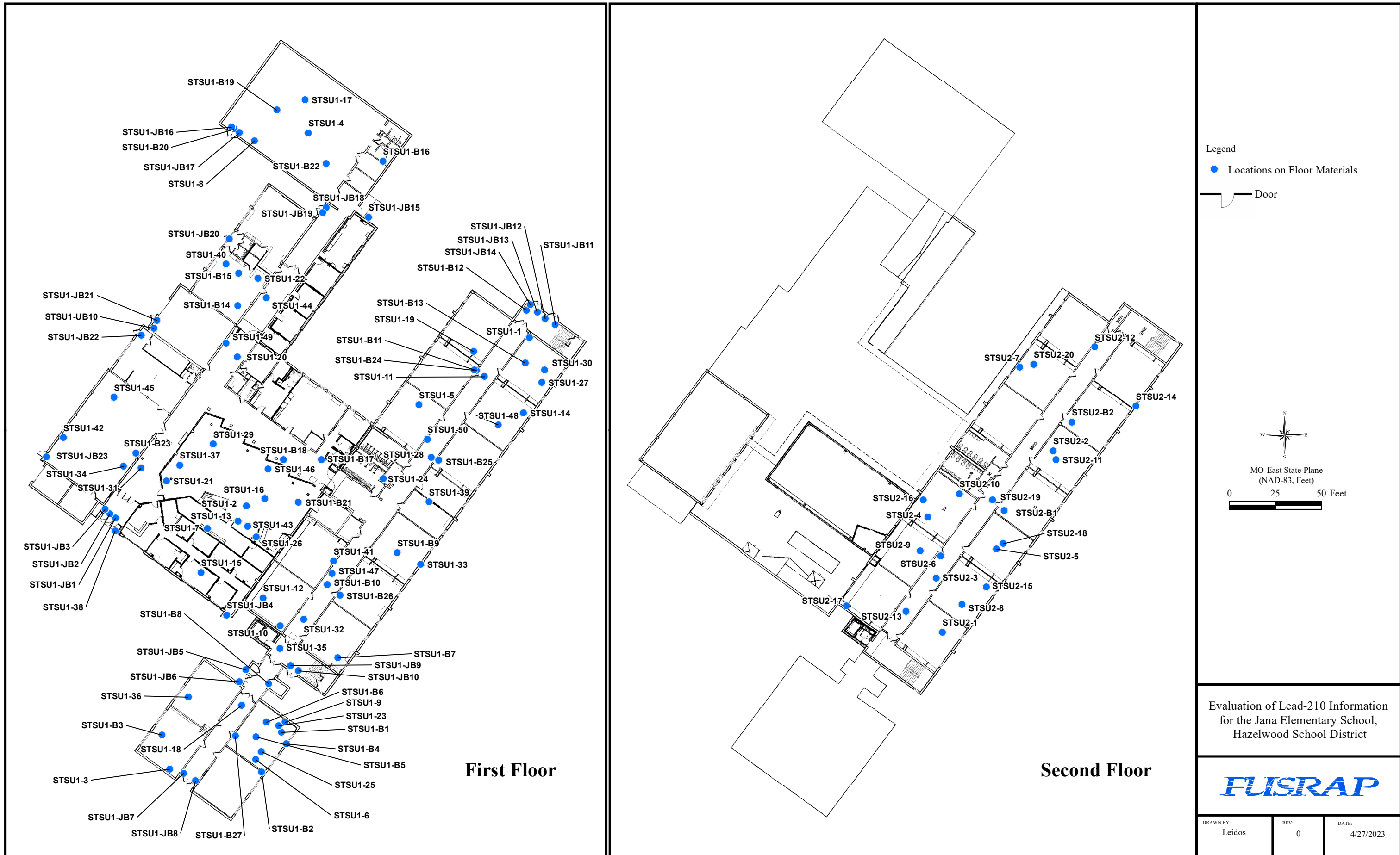
Figure 5. Structure Surface Survey Locations for Floor Materials
