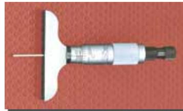
The depths of holes, slots, shoulders, and projections can be measured to .001" or 0.01mm with these fine tools.
