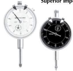
These Indicators are graduated in .001" or .01mm with the second hand reading every .010" or .1mm. Range per revolution .10" or 1.0mm. Reading 0-100. Back has clamping lug.
