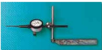
Shown with detachable deep hole attachment held in tool post holder with upright spindle and snug, complete.
