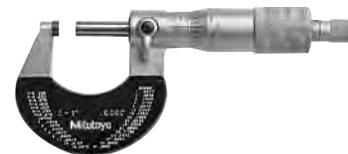
102 Series Micrometers are the deluxe version of the 101 Series. A pair of black heat insulating grip plates are attached on the frame. The micrometer comes with a friction thimble or ratchet stop to assure consistent measuring pressure, and reduce discrepancies in final readings from one inspector to another. The friction thimble has a speeder to quickly open and close the spindle.
