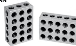
Used in layout and setup work. Each set consists of 2 matched, hardened and precision-ground blocks. The squareness on all sides is within .0001" per inch. The blocks are supplied with a plus allowance of .0001" to .0003" to allow nominal lapping. Five 3/8"-16 tapped holes are provided for clamping. SUBURBAN sets include wooden case.
