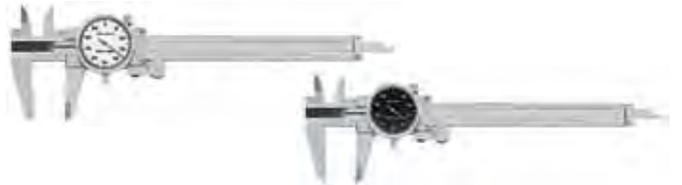
Of stainless steel, hardened throughout with satin-chrome finish. Suitable for outside, inside, depth and step measurement. Thumb roll. Direct reading in .001" or .02mm with adjustable dial setting and locknut. Covered rack for longer life. Fitted case. .100" or 2mm per revolution.
