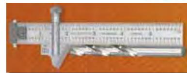
Provides a quick accurate way for determining the correct drill point angle of 59° and the correct length of drill lips.
