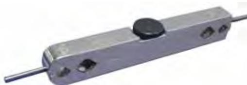
Handles all Plug Gage sizes from 1/32" thru 1/2", 0.79 to 12.7mm diameter. GO and NO-GO clearly marked.
