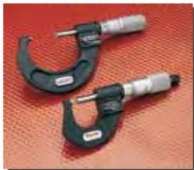
Digital micrometers make readings faster and easier. Thousandths of an inch are read directly from a counter. Ten-thousandths of an inch are taken from a quick-reading vernier scale on the micrometer sleeve. The frame-mounted counter saves considerable handling time since its numbers can be read without removing fingers from thimble or micrometer from hand.
