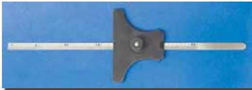
Head is made of hardened steel with protractor graduations in 30°, 45°, and 60° angles. The base surface measures 2-1/2" x 1/8" thick. The 6" rule has 32nds or mm graduations on one side and 64ths or 1/2mm on the other side. A 6" rod is included for measuring depths in narrow places.
