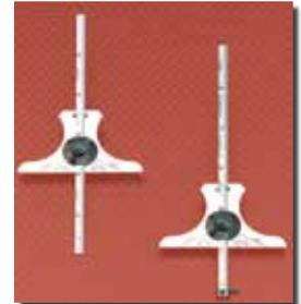
Can be used as depth gage by simply reversing the rule, as protractor for measuring 30, 45 and 60 degree angles and, if rule is removed, it can be used separately. Hardened, polished steel head measures 2-5/8" (66mm) long x 1/8" (3mm) thick. Steel rule can be locked in any position.
