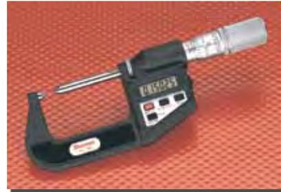
Micrometer has 60 degree conical anvil and spindle faces with 1/64" (0.4mm) flats on the ends of the points. This allows measuring in small grooves, recesses, and many other applications that conventional micrometers are not suited for. (Will not measure pitch diameter).
