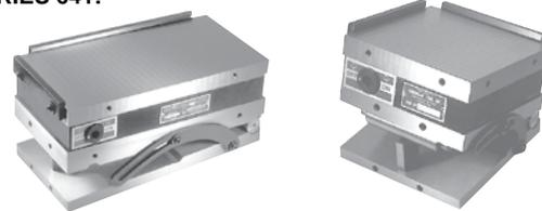
Ceramic permanent magnetic chucks can't lose their magnetism. Removable handle for ON/OFF operation, end rail and side rail all included. Sine plate angles lock rigidly with locking strap. Squareness, parallelism and roll center distances within .0002" and .0003". Unit features .200" minute angle steps.
