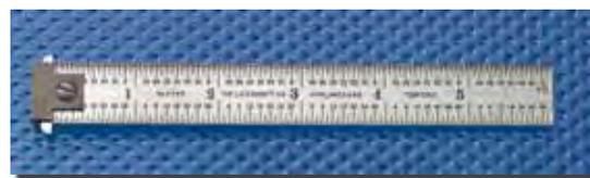
Convenient hook rule permits accurate measurements even when the user cannot see if the rule is even with the measuring edge. Especially useful for measuring from round corners, through hubs, for setting inside calipers, etc. The single hook is hardened and may be reversed or removed entirely. Rule made of high quality steel, satin chrome finish, machine-divided graduations.
