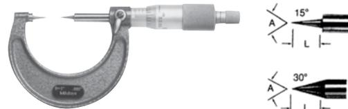
For measurements of small grooves, keyways and other hard-to-reach dimensions. The measuring points have approximately .012" radius, and are available with or without carbide tips.
