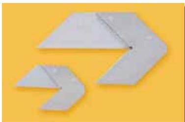
Similar to Starrett hardened squares except that blades are beveled on both edges of each side, providing practically a line contact with work. Beam and blade are hardened, ground and lapped to insure parallelism and straightness. The beam is grooved at inner corner for clearance of burr and dirt.
