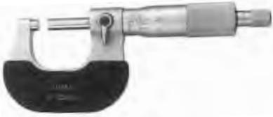
MEDA micrometers from 0-1 through 3-4 have forged steel frames and plastic insulating plates; micrometers from 4-5 through 11-12 have lightweight enamel frames.
