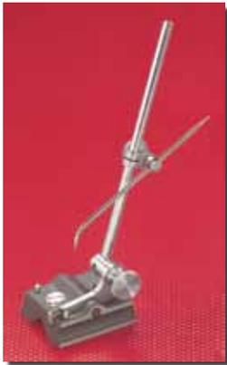
Standard size for all-around work. Cast base with black wrinkled finish. Ground bottom surface, polished sides, two gage pins for linear work, and V-groove for cylindrical work. Spindle adjustable to any angle above or below work. Scriber may be used in small hole in place of lower sleeve in place of spindle. Fine adjusting screw in base rocker.
