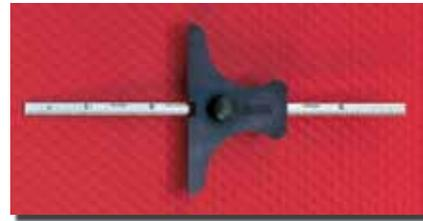
Consists of case hardened steel head, 2-5/8" long by 1/8" thick / 66 x 3mm, and 6"/150mm tempered steel rule fitted to slot in head. Rule locked in position by knurled nut and friction spring.
