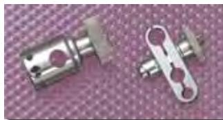
Adapts indicators or scribers to surface gages and other tools. Sleeves provide a convenient means of attaching scribers and indicator shanks to surface gages, magnetic bases, indicator tool post holders and gage rods. The large diameter knurled clamping nut provides a firm grip on rods, posts and scribers.
