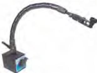
Strong magnetic holding power includes "V" area for clamping to round surfaces. On/off switch, made of hardened and ground components, flexes almost 360°, and is rigidly locked into position with a lever. Includes 5" rod having 3 different diameters and a swivel adapter for lug back indicators to accept all AGD dial indicators.
