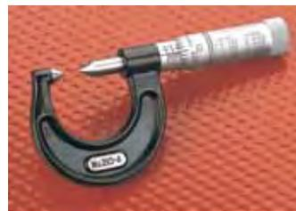
Designed for comparing threads, measuring in grooves, recesses and other applications. (Will not measure pitch diameter.) Conical anvil and spindle faces with 1/64"(0.4mm) flats on points. Black enamel frame. Satin chrome finish on sleeve and thimble. Hardened threads ground from the solid. Fitted Case. No Ratchet or Lock Nut
