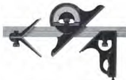
Hardened and Ground. Set includes 12" stainless steel chrome plated blade with 4R inch (8ths, 16ths, 32nds, 64ths) graduations, double indexed and reversible Protractor Head with full 180° graduation and spirit level, Square Head with level and scribe, and Center Head.
