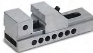
All surfaces hardened and precision ground to ± .0002". Base and stationary jaw are one solid piece. Horizontal and Vertical "V" on moveable jaw for holding round work. Up to 400 lbs. pressure at 45° downward angle keeps work rigid. Quick adjustment is made by pulling pin and pushing sliding jaw forward -then tightening with an Allen wrench.
