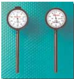
Back plunger indicators include a 3" (75mm) detachable deep hole attachment interconnecting directly with the main spindle for positive action. The attachment is for checking internal dimensions of a workpiece while in fixtures or machines and can be easily removed.
