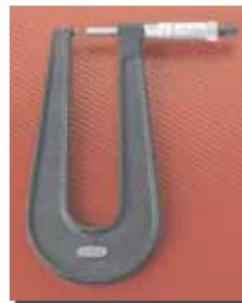
These micrometers reach over the edge of sheet metal and take measurements away from the edge toward the center. Also for other gaging jobs where a deep throat micrometer is needed. Rounded anvil on 1"/25mm size gives a point contact for more accurate gaging; flat anvil also available. 1/2"/ 13mm micrometers have Satin Chrome Finish; 1" micrometer frames have black wrinkle finish.
