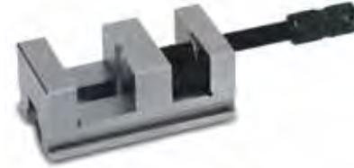
Made of hardened steel. All surfaces including jaws are precision ground with .0004" accuracy for flatness, parallelism and squareness. Can be used in any position. Models 1730001 and 1730002 have "V" grooved jaws for holding round work.
