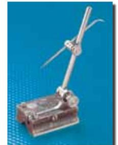
Smaller size ideal for lighter work. Hardened steel base, ground and polished, with two gage pins for linear work plus V-groove for cylindrical work. Spindle adjusts to any angle above or below base. Scriber and spindle holes are in permanent alignment, and scriber may be used in small hole of lower sleeve in place of spindle. Knurled thumb screw in base rocker provides fine adjustment.
