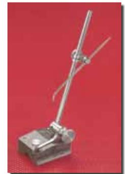
Hardened steel base with ground and polished contact faces, four gage pins for linear work, and V-groove for cylindrical work. Spindle adjusts to any angle above or below base. Knurled thumb screw on base rocker for extra fine adjustment.
