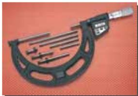
Each micrometer is equipped with a series of easily interchangeable anvils, thus providing the full range in steps of one inch with a single micrometer. Suitable wrenches are furnished to make necessary adjustments. The larger sizes have .300" (7.6mm) anvil and spindle diameters for ease of use on larger work.
