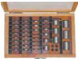
Can often take the place of gage blocks. Outside diameter is .750"; inside diameter has 1/4" - 28 thread for accurately connecting the individual blocks. 4 threaded connecting studs included. Hardened, ground, and lapped to ±.0001". Supplied in fitted wooden case.
