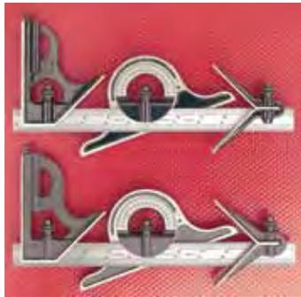
With reversible lock bolts, scribe, spirit level in both square head and protractor head. Direct reading double 180° protractor scale, and hardened steel machine-divided blade. Cast Iron Heads with black wrinkle finish.
