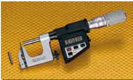
Interchangeable anvil micrometer permits quick, accurate measurements of tubing, cylindrical walls, from a hole or slot to an edge, and in many other hard-to-reach places. Two anvils are furnished with the tool – a round anvil, approximately .120" diameter; and a flat anvil, approximately .125" diameter and .060" in thickness. Anvils are rigidly held in a vise-type frame that allows for quick changes by a single lock screw.
