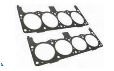
**A. Composition Material Cylinder Head Gaskets** Thick, 0.040" to 0.042" Composition Material Cylinder Head Gaskets can be used for competition applications up to 12.5:1 compression ratio. Sold as an engine set. Small Block 4-bolt pattern.
