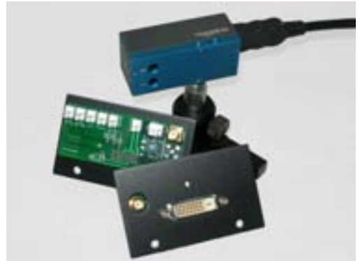
Figure 1.1: The MOGlabs DLC is readily connected to a laser diode, temperature sensor and thermo-electric cooler via the provided laser head board.
