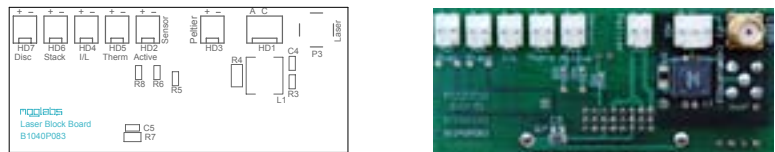
Figure F.1: MOGlabs DLC laser head board showing headers for connection of laser diode, piezo actuators, temperature sensor, TEC and head enclosure interlock.
