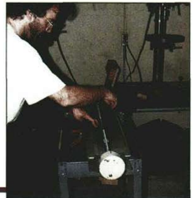
Case sides begin life as flat sheets of plastic. Corners are carefully bent by hand, using a heating element rod.
