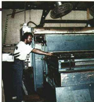
This sizable machine vacuum-forms literally dozens of sizes of lids and bottoms for Impact's plastic cases.
