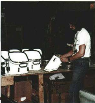
Toms with cutaway designs and Impact's unique "sound holes" are used in marching limp-toms and on some drumkits.
