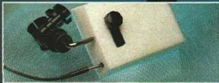
Igniters mount on standard Tama pencil mounts and connect with a 1/4" phono plug.
