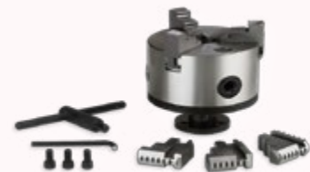
005-0040 Self-Centering 3-Jaw Chuck Includes two sets of manually adjustable jaws from 7/8" - 3 3/4" internal and 1/8" - 4" external clamping.
