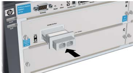
Figure 7. Installing an X2 transceiver
