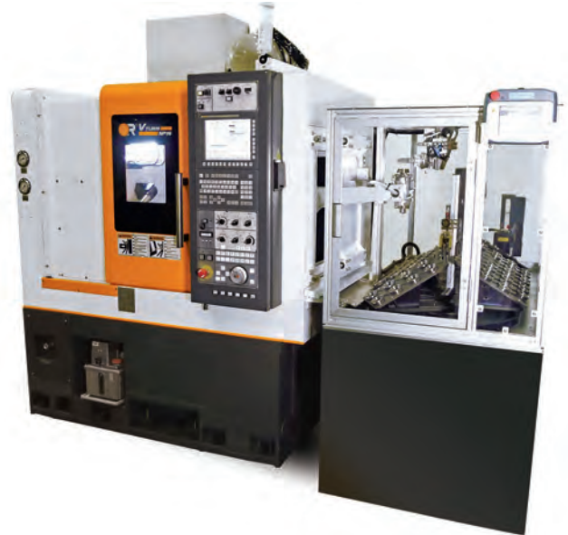
A single Victor Vturn-NP16 turning center with a robot system and pallet changer
