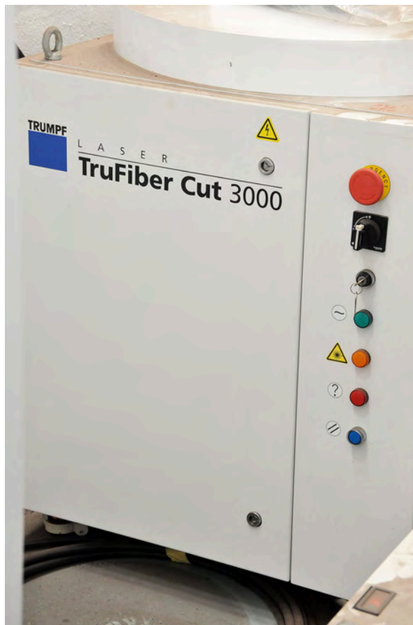
The JFY fibre laser is powered by a Trumpf TruFiber Cut 3000 source
