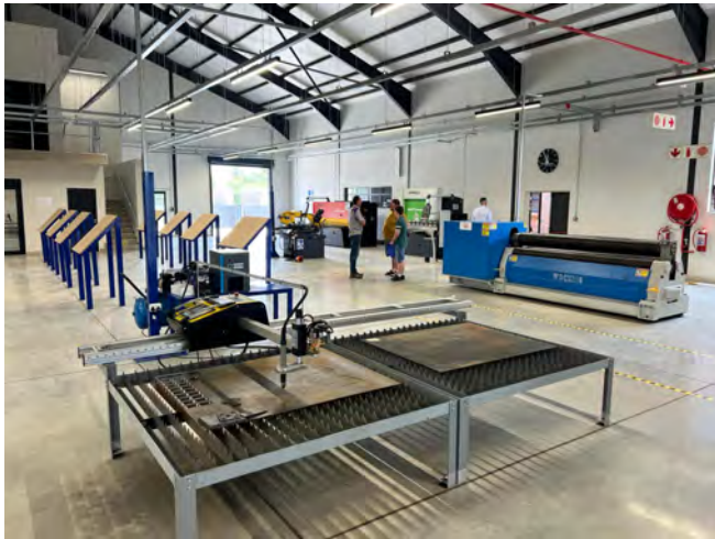
The forming side of metalworking is covered with a CNC plasma cutter, a guillotine, a press brake and a plate rolling machine, all supplied by TH Machine Tools
