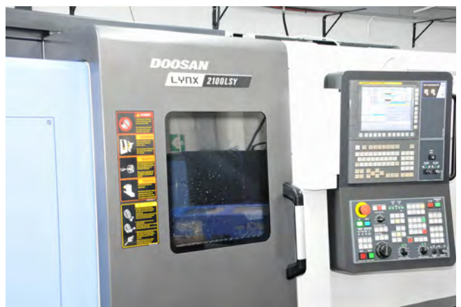
One of the CNCs on the shop floor is a Doosan (now DN Solutions) Lynx 2100LSY CNC horizontal turning center, supplied by Puma Machine Tools
