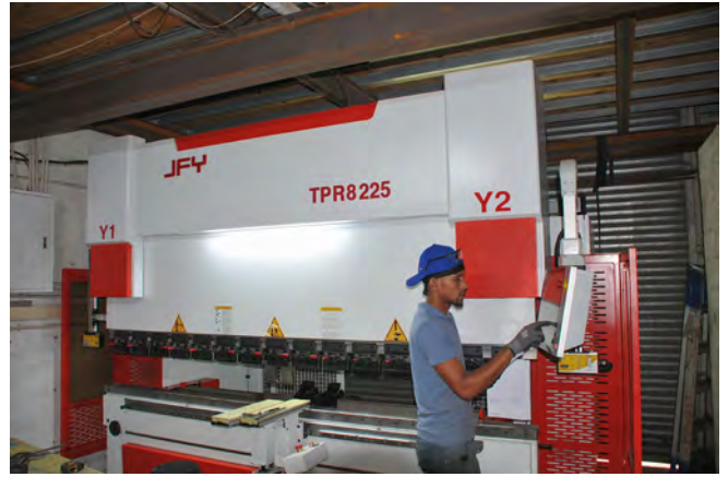
The company has recently purchased a JFY TPR 8225/3100 CNC press brake which has a mouth of 3 100mm and a press force of 225 tons. This machine was supplied by Puma Machine Tools
