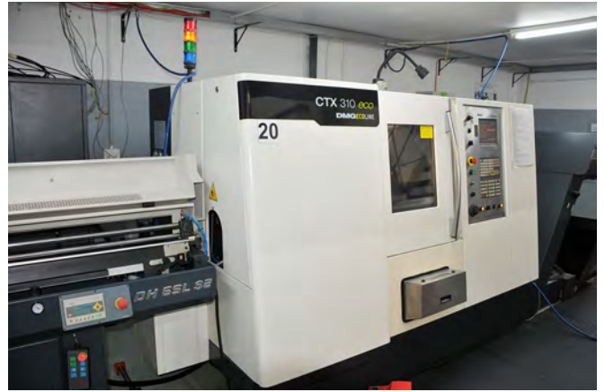
Another of the CNCs on the floor is a DMG MORI Ecoline CTX 310 lathe
