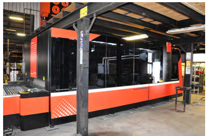
In 2023 Technipunch CC added a further two fibre lasers to the floor with the latest purchase only being installed late last year. The DNE is a 6kW laser and has a bed size of 4m by 2m
