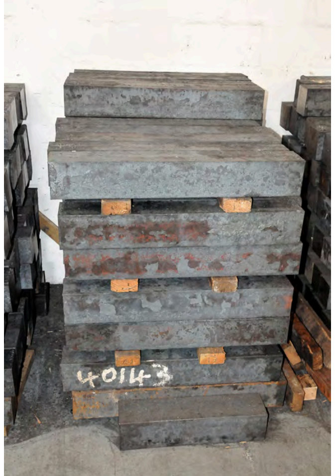
Counterweights are typically made of steel, iron, or concrete and the battery alone can weigh anywhere between 240kg to 2500kg
