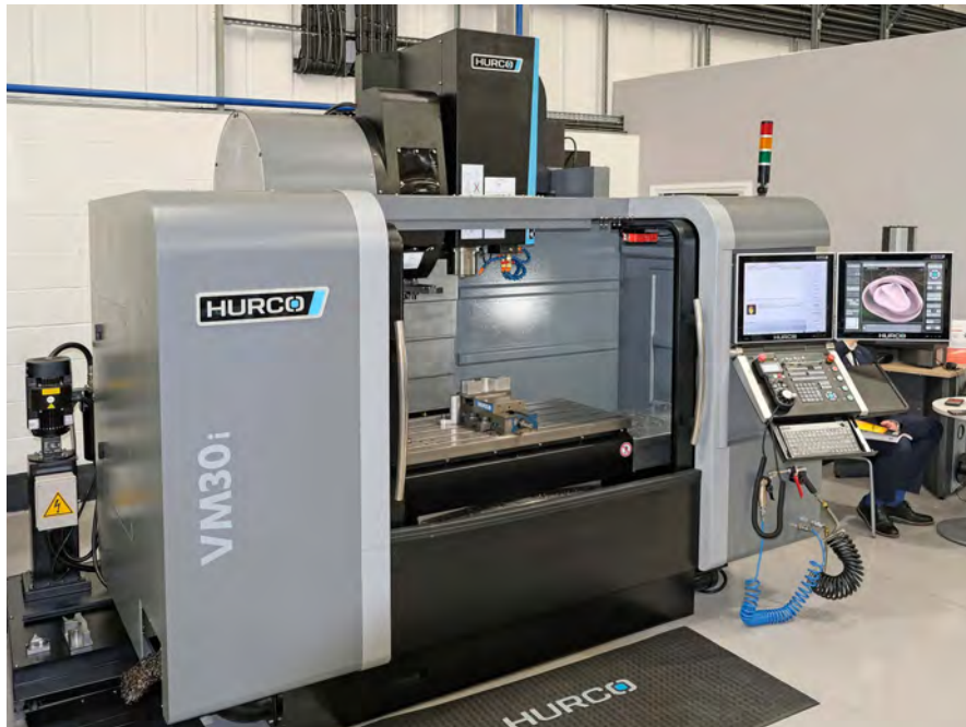
The machine now includes a twin- rather than single-screen control
