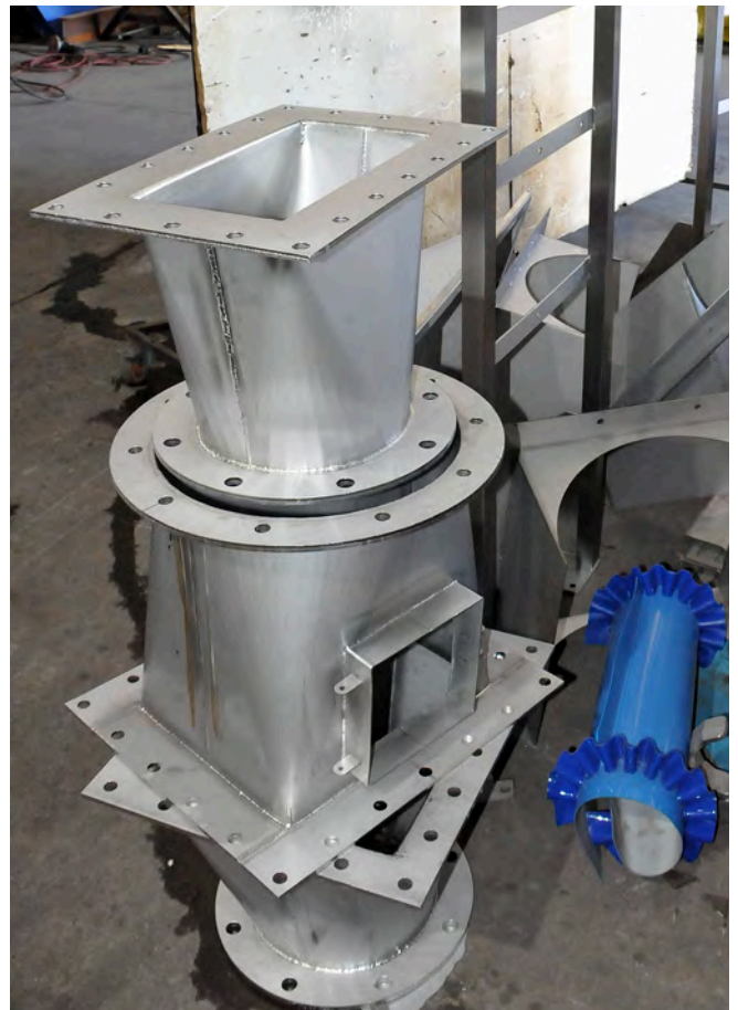
Various components that have been manufactured to replace wear parts
