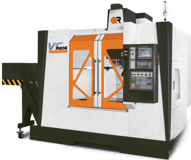
The popular Vcenter-P106 includes rapid feeds of 48/48/32m/min, 12 000rpm, spindle output of 18.5kW, BBT 40 / 30 tools, roller guideways, bottom guarding flush and screw chip remover
