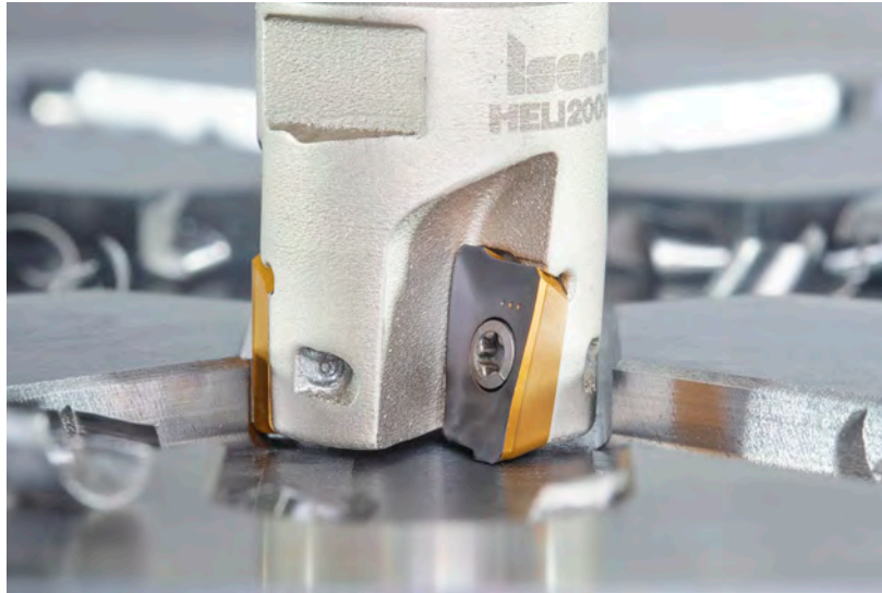
Fig. 1 A typical Helimill insert: a helical cutting edge is formed by the intersection between the helical side and the shaped top surfaces of the insert
