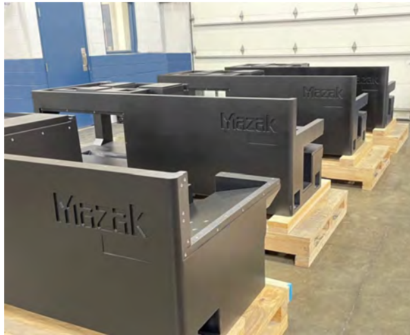
The photo shows mineral casting used in the Syncrex Swiss-type CNC automatic lathe manufactured in the United States
