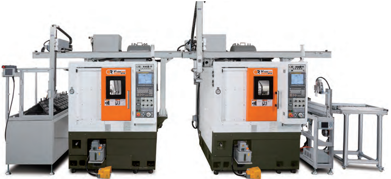
For flexible automated production, Victor CNC can integrate the EWR-03 articulated robot system that can tackle parts weighing 3 kilograms of dimensions up to 120mm diameter. Part loading/unloading time can be just seven seconds
