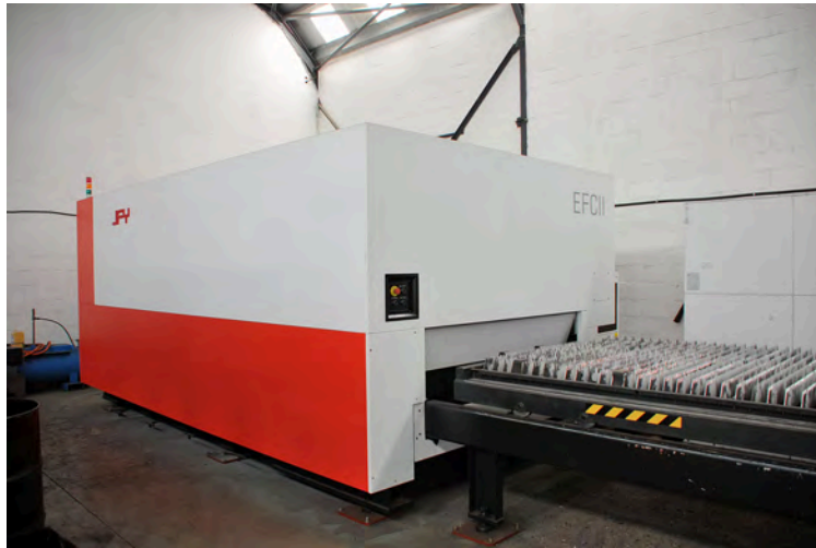
A fibre laser was Trax Engineering’s first major equipment investment. They purchased a JFY 3kW with a 3m by 1.5m bed from Puma Machine Tools that was installed in August 2023
