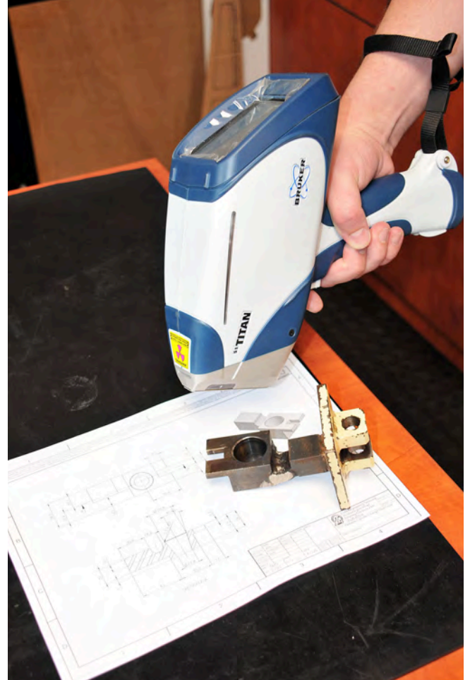
LEDA rely on a handheld Bruker XRF analyser that enables them to perform rapid and accurate material analysis in-house
