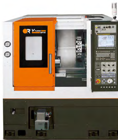
The cover image features Victor Taichung’s robust Vturn-NP16 turning center, which boasts a compact footprint of just 1 488mm in length by 1 956mm wide, and has a height of 1 775mm, Z-axis travel of 250mm, a 570mm diameter swing-over-bed and a 260mm maximum turning diameter
