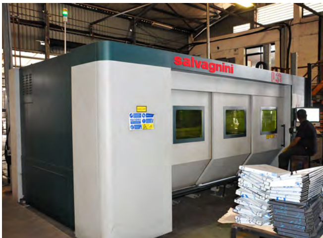
“After initially purchasing our first fibre laser – an Ermaksan Fibermark – in 2015, which is still running, we only purchased our second one in 2019. The Salvagnini is a 6kW fibre laser and we added entry level automation to it.”
