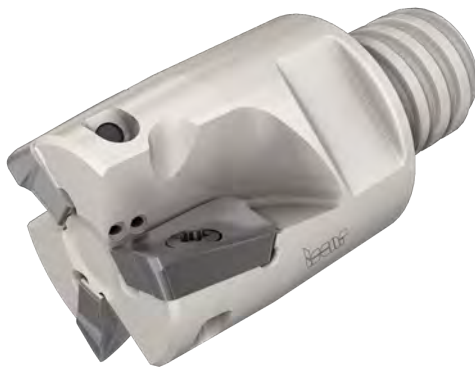
Fig. 3 An exchangeable milling head carrying rectangular-shaped inserts with HPC option. Decreasing chip gullet enables increasing tooth density
