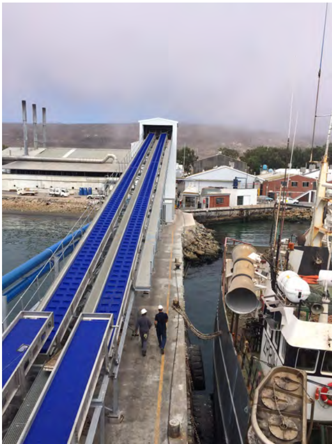
Conveyor systems are one of Leading Edge Engineering’s specialties. This one is used for off-loading fish from the boat
