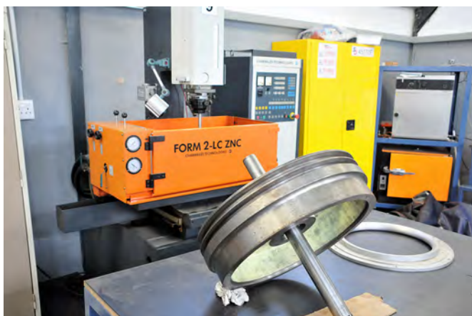
Components are not always small and intricate with large production runs, one-offs and machine specific components are also a feature. The LEDA Group uses their EDM machine where necessary
