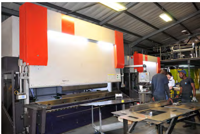
In the press brake department Technipunch have installed two Bystronic machines. One is a 250 ton by 4m and the other is a 150 ton by 3m
