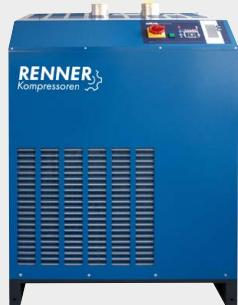
The all-in system for compressed air treatment comes with a dew point indicator, metal housing and power plug. The aluminium heat exchanger has three functions: it serves as air-to-air heat exchanger, as air-to-refrigerant heat exchanger and condensate drain.
