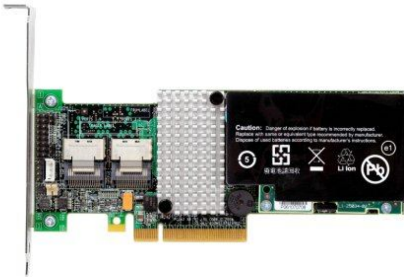
Figure 7. IBM ServeRAID M5015 SAS/SATA Controller with the battery backup unit attached
