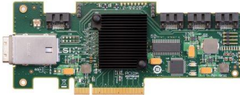
Figure 15. IBM 6Gb SAS Host Bus Adapter with the PCIe slot bracket removed
