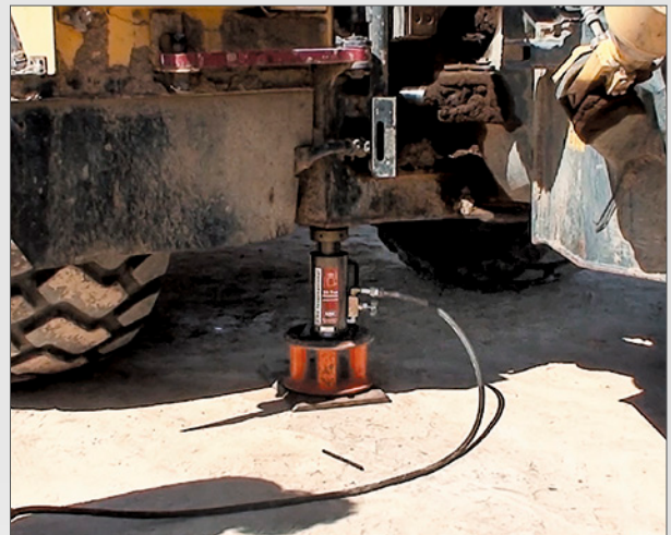
The 55-Ton Load Lock'R Aluminum Jack in use.
