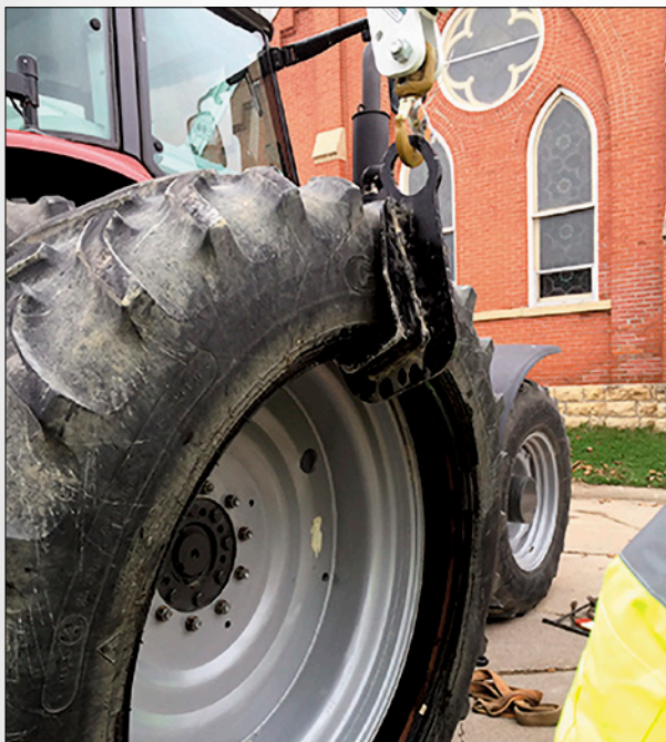
The Earthmover Tire Bead Hook in use.
