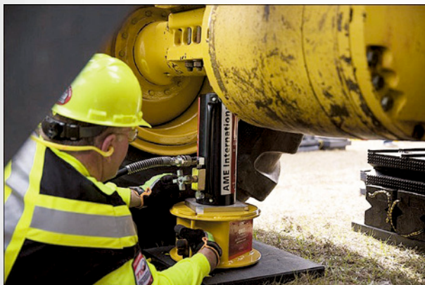
The Steel Crib Stand in use.
