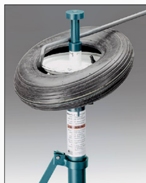
The Floor Mount Manual Tire Changer in use.
