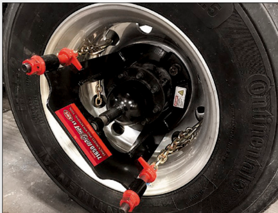
The Truck Wheel & Rim Removal Tool in use.
