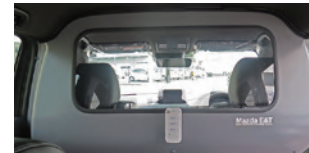
A partition wall installed between the front and second row seats
