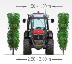
From 1.5m width, ideal for more extensive vineyards & fruit orchards with rows from 2.5 to 3.0m. A more substantial tractor with a wider front axle and a more spacious cab.
