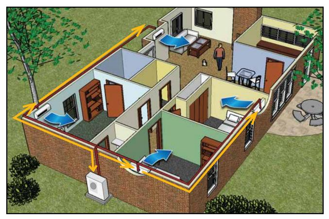
You can see how one outdoor condenser is used in conjunction with multiple indoor air handlers in a single structure. Air handlers can be installed up to 115' (depending on model) from the condenser, so you can place the condenser in the best location for your landscaping.
