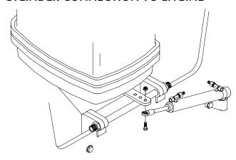
HC5380-3 SPLASHWELL CYLINDER TYPICAL SINGLE ENGINE MOUNTING
