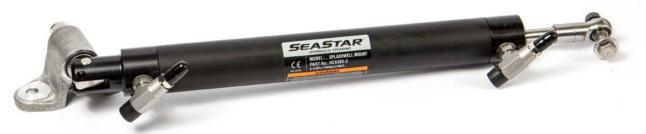
This cylinder is a light duty alternative to front & side mount cylinders. It is unbalanced with 5.5/6.5 turns lock-to-lock and fits engines with/without support (steering) tube. The splashwell mount cylinder is for single & multiple engine capability and has total power to 600 HP in counter rotating application. It can be transom or hull mounted cylinder. NOTE: Not for use with SeaStar Pro helms.
