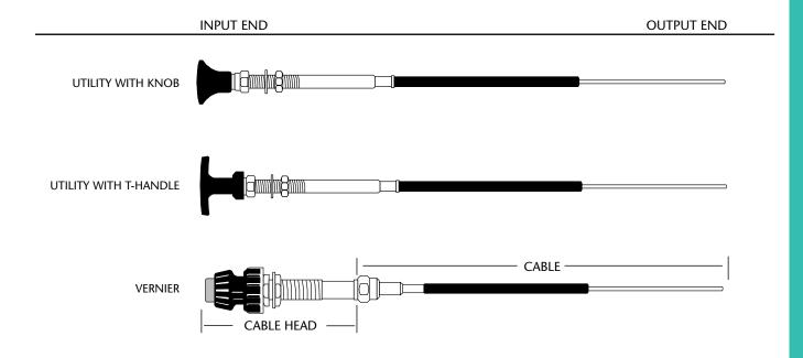
Note: The Marine Utility and Vernier control cable has a bare conduit at the output end with a .075 stainless steel wire.
