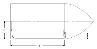
A single-cable, starboard drive push-pull mechanical cable system is shown in this diagram. If your mechanical system is different than the one depicted and/or you have any questions about mechanical steering after reviewing this guide, please contact SeaStar Solutions Technical Service.
