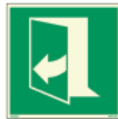
Door opens by pulling on right-hand side [MES009]
