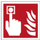
Fire alarm call point
