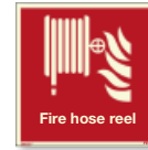
Fire hose reel [FES002]
