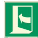
Push door on left-hand side to open [MES011]
