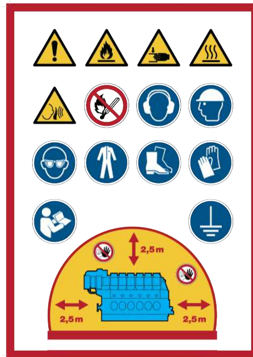
Figure 90: Warning sign E11.48991-1108
