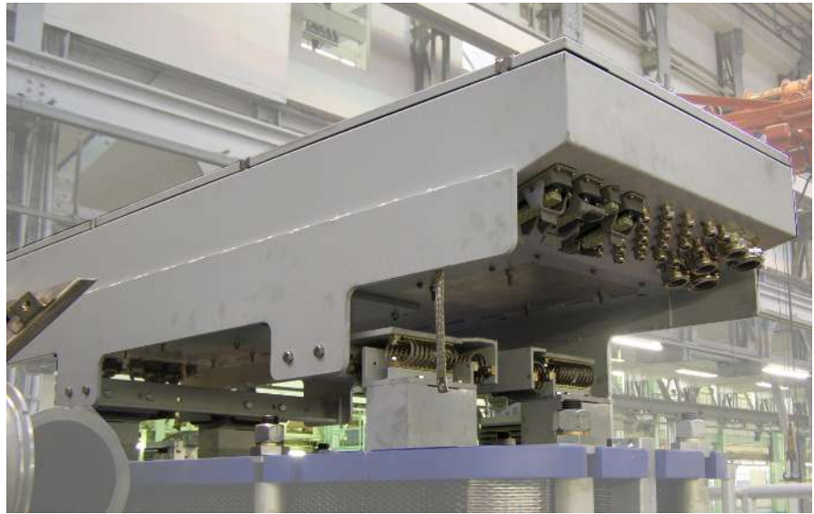
Figure 41: Control and Injection Unit
