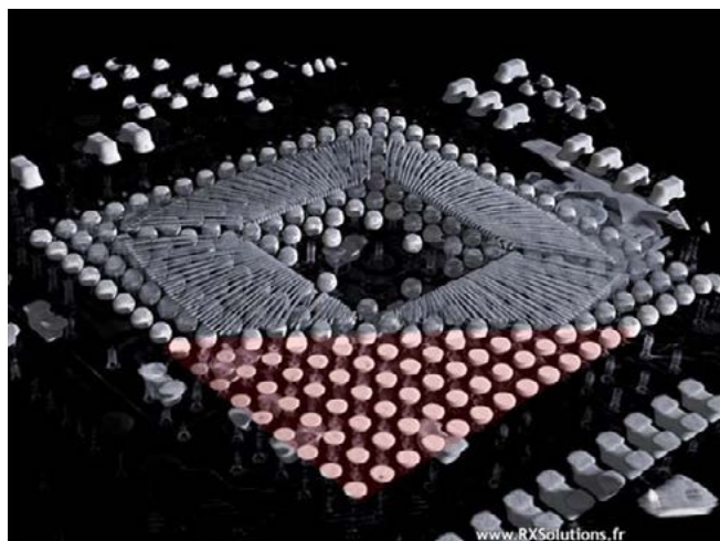
Figure 6: CT reconstruction of a BGA package using micro CT reconstruction from a very large number of images.
