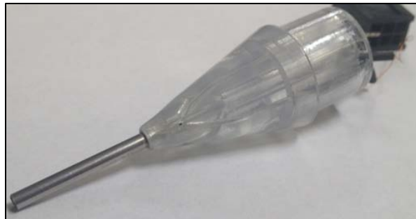
Figure 4: A photograph of the prototype of the cone tip and thermal conductivity.
