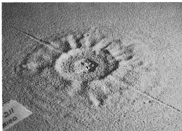
Figure 3. Hummocky Mounds and Concentric Rings Surrounding Crater Produced in Layered Media with Shallow Overburden.
