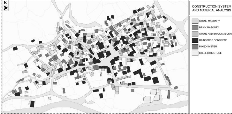
Figure 5. Construction System and Material Analysis.
