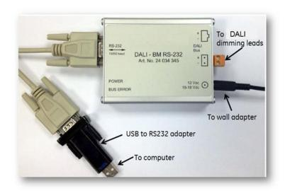
☐ **The DALI programmer** TRIDONIC.USA DALI-BM RS-232 Art. No. 24 034 345 with a USB to RS232 adapter. Direct Ordering information:
