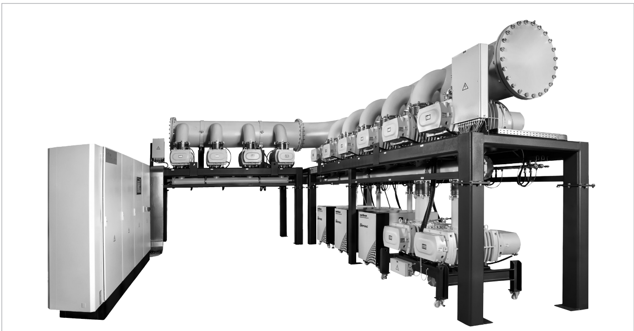
Pump system for the field of steel degassing
