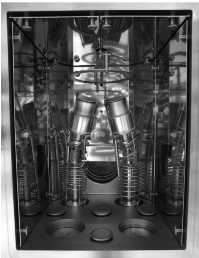
Two magnetron sputter sources, confocal aligned to the substrate holder rotating at the chamber top. Spare flanges for two further sputter sources
