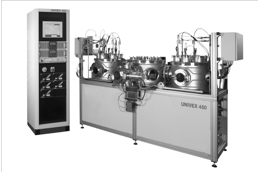
Design example: UNIVEX 450 C with coating module and electrical cabinet (example photograph). The coating module consists of two process chambers (left and right) as well as the loadlock and transfer chamber in between The substrate transfer between the chambers is effected with the aid of a vacuum robot
