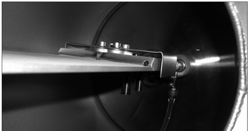
Insulated substrate fork with RF bias connection
