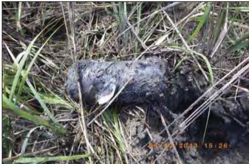
Flare, Aircraft, LUU-4B, Expended (north of AOI A) (4/24/13)
