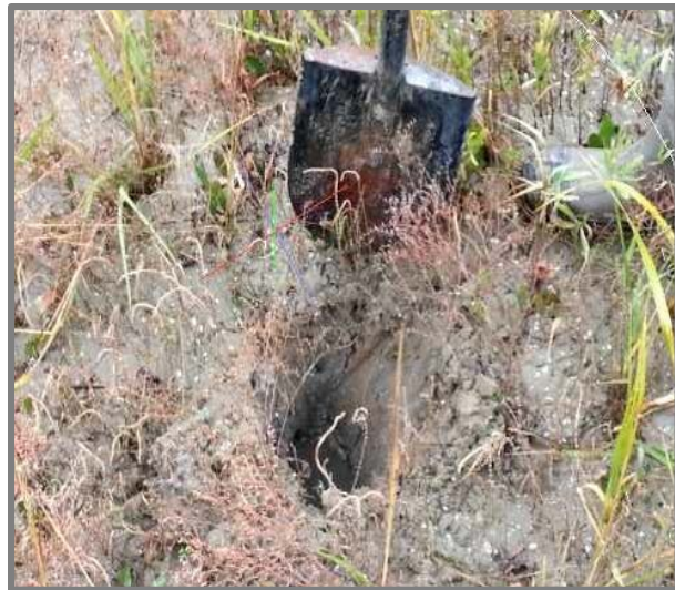
Test Hole in Dry Sands of Upland Areas
