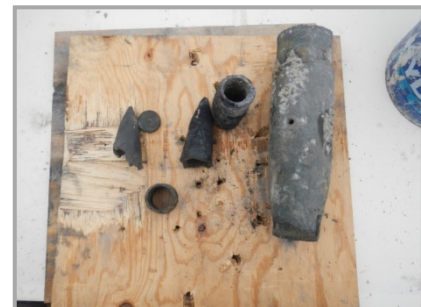
Two 2.75-inch and one 5-inch Practice Rocket Warheads, Post-detonation
