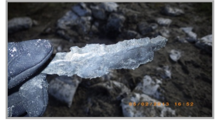
Metal Fragment Found in Pit After Detonation of the HE-filled, 5-inch Rocket Warhead
