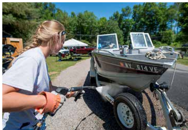
Watershed Stewards decontaminating watercraft at Back Bay on Upper Saranac Lake utilizing Upper Saranac Foundation's, high pressure, hot water decontamination unit.
