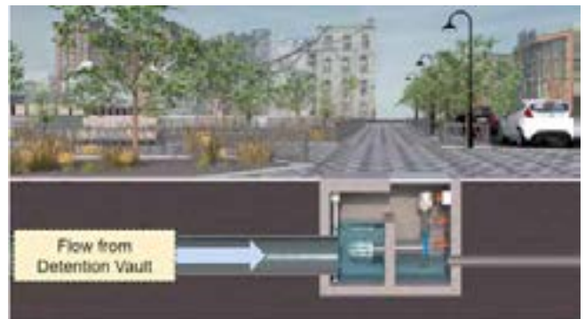
Rendering of a CMAC actuated valve used for CSO-mitigation at Southwest Park in Hoboken, NJ.
