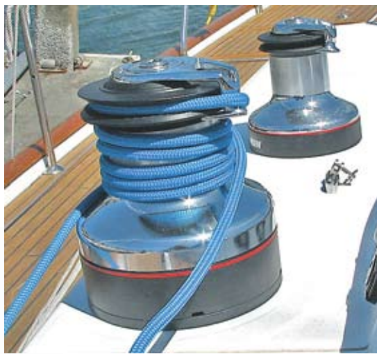
You never really need this many turns on a winch. At five turns, 10 lbs of tailing force would hold over 25,000 lbs of sheet load.
