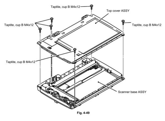
(5) Remove the six cup B M4x12 Taptite screws, and then remove the top cover ASSY.
