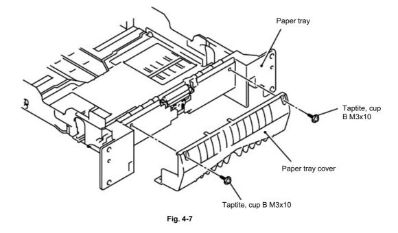
(5) Remove the two cup B M3x10 Taptite screws, and then remove the paper tray cover.
