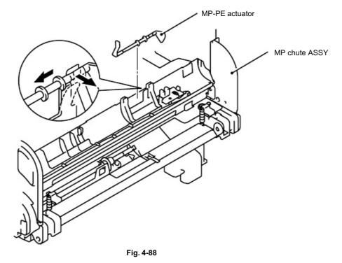
(14) Remove the four bind B M4x12 Taptite screws, and then remove the MP chute ASSY.
