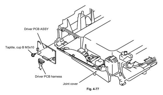
(8) Remove the cup B M3x10 Taptite screw, and then remove the driver PCB ASSY.
