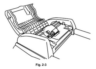
(2) Slide ADF support into the groove on ADF.
