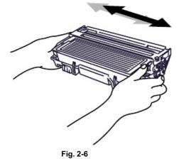
(4) Push the drum unit assembly into the machine (until it snaps into place).
