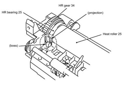
When re-assembling the heat roller 25 to the FU frame upper, ensure you do not damage • the heat roller 25 with the four separate claw ASSY on the FU frame upper.
