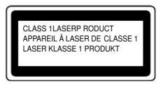
This printer has a laser diode which emits invisible laser radiation in the Laser Unit. The Laser Unit should not be opened without disconnecting the two connectors connected with the AC power supply and laser unit. Since the variable resistor in the laser unit is adjusted in accordance with the standards, never touch it.
