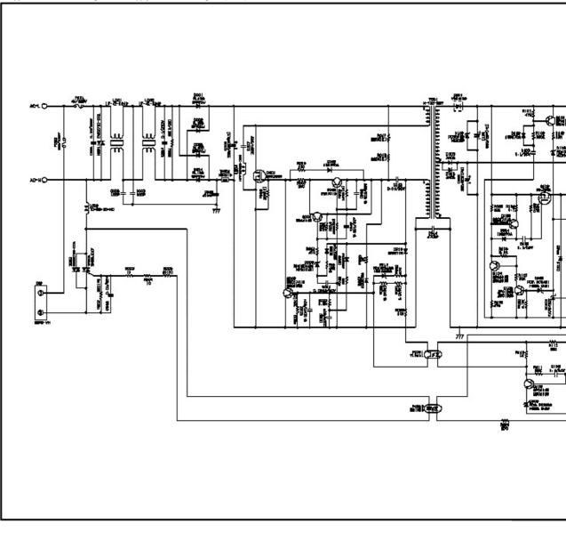
Appendix 4.17 Low-voltage Power Supply PCB Circuit Diagram (100V)
