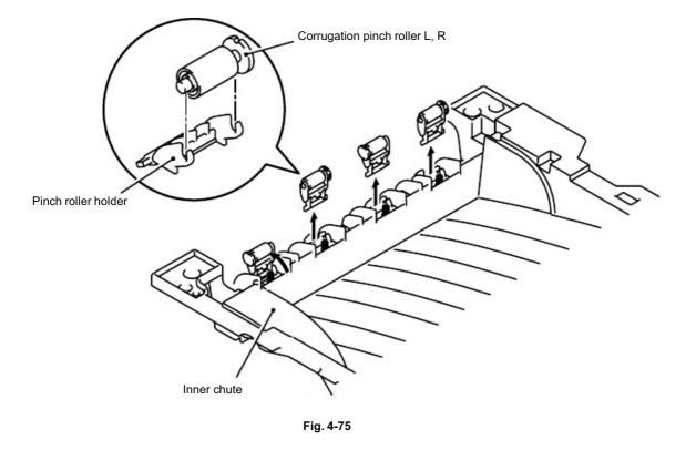
(5) Remove the corrugation pinch roller L, R and pinch roller holder.
