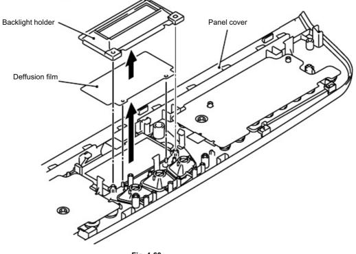
(5) Remove the backlight holder and the deffusion film.
