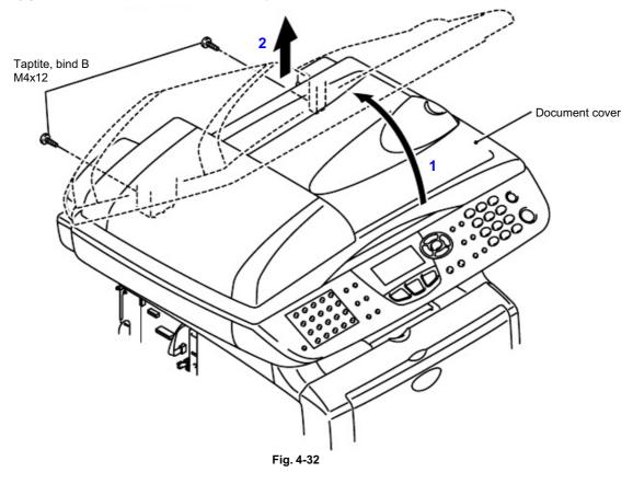
(4) Remove the two bind B M4x12 Taptite screws, and then remove the document cover.
