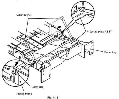
(16) Unhook the pressure plate spring from the plastic hook to remove the two pressure plate springs.
