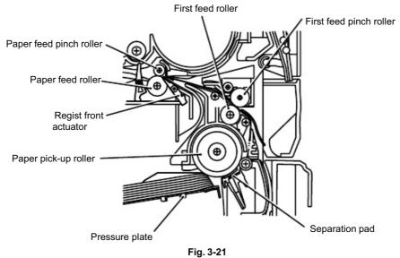
The paper is gripped between the paper pick-up roller and the separation pad and separated into individual sheets.
