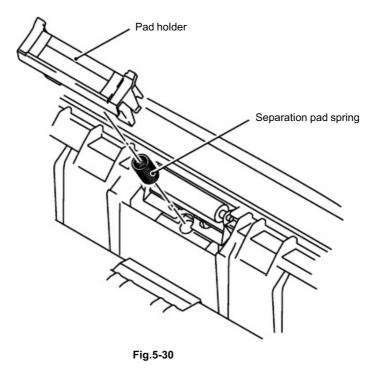
3) Remove the pad holder and the separation pad spring from the paper tray.
