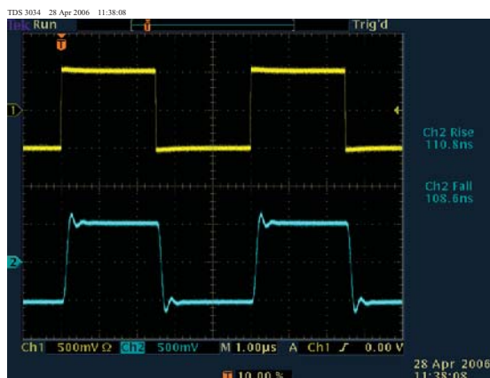
Figure 4.1: Response of the SIM983 to a 1.0 V peak-peak step, G = +1.00 , V_{ofs} = 0.000 V.
