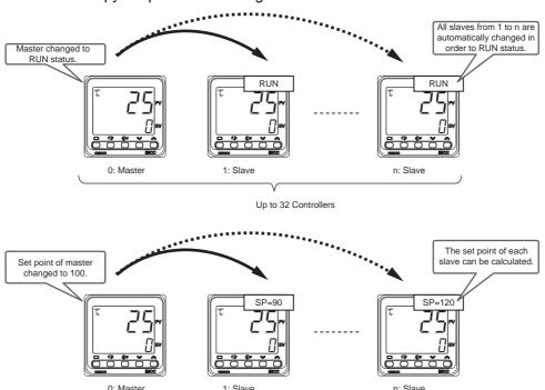
Note: To use component communications, the input type and, if an analog input is used, the decimal point position must be set to the same values for all of the E5 C Controllers. The operation will not work correctly if the position of the decimal point is different.
