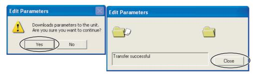
Click the Yes Button to restart the Unit. Select All ports and then click the OK Button. A dialog box will be displayed when the Unit has been restarted. Click the OK Button. This completes the PLC setup procedure. You will use the CX-Programmer to check operation, so leave it online.
