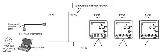
Note: Refer to the KV STUDIO User's Manual for the installation procedures for the KV STUDIO and USB driver.
