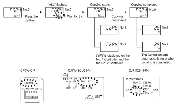
For a Mitsubishi PLC, the ERR. indicator on the Serial Communications Module will light during the copying process. Ignore it and check the operation. The ERR. indicator will go out when the PLC is restarted.
