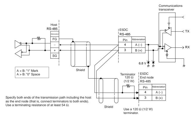
Match the communications specifications of the E5□C and the host. When using a 1:N connection, set the same communications specifications in all of the Units. Each Communications Unit must have a unique unit number.
