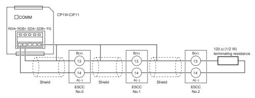
Note: 1 The maximum transmission distance is 50 m for the CP1W-CIF11 and 500 m for the CP1W-CIF21.
