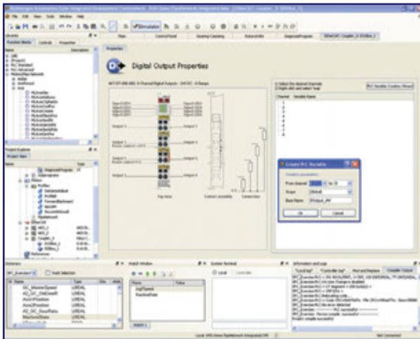
Automatic I/O variable creation with scope definitions Adding bus couplers with I/Os onto a motion network topology
