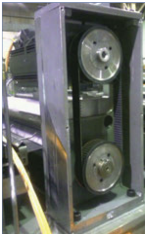
Press feed machine built with a conventional servo motor, gearbox, belt and pulleys.
