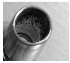
Fig. 3 Nozzle appearance after 40 minutes continuous of welding
