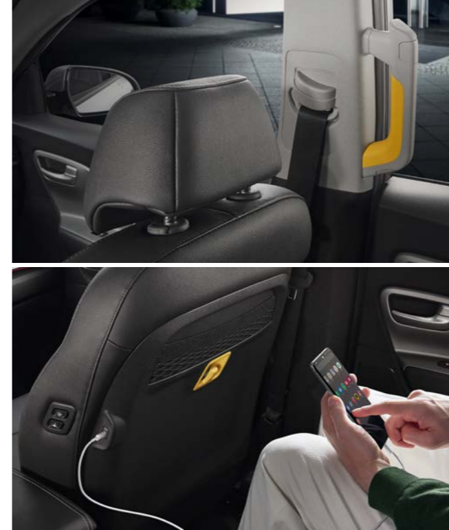
Slim passenger-seat headrest (Taxi model) / B-pillar assist handle A slimmed-down headrest on the passenger seat offers 2nd-row passengers a greater sense of space and a wider forward view. B-pillar assist handles help passengers get on and off the car easily.
