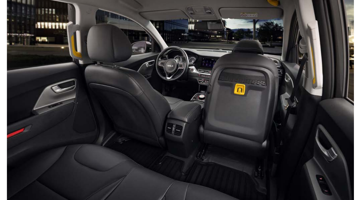
2nd-row seatbelt buckle illumination (Taxi model) / 2nd-row door reflectors LED lighting on seatbelt buckles increases visibility to help occupants fasten their belts. Reflectors on 2nd-row door armrests help passengers to get on and off the car safely.
