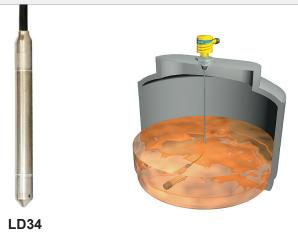
The general purpose LD34 small-bore submersible pressure level transmitter provides continuous level measurement up to 100' (30.4m) of water column with a 4-20 mA signal output. Select the LD34 liquid level sensor for relatively clean water. Application examples include ballast tanks, ground water monitoring, surface water monitoring, dewatering, down hole, and remediation.
