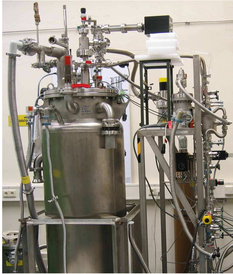
Figure 41: TRAP experiment. Shown are the cryostat with inserted tube (left) and the gas handling system (right).
