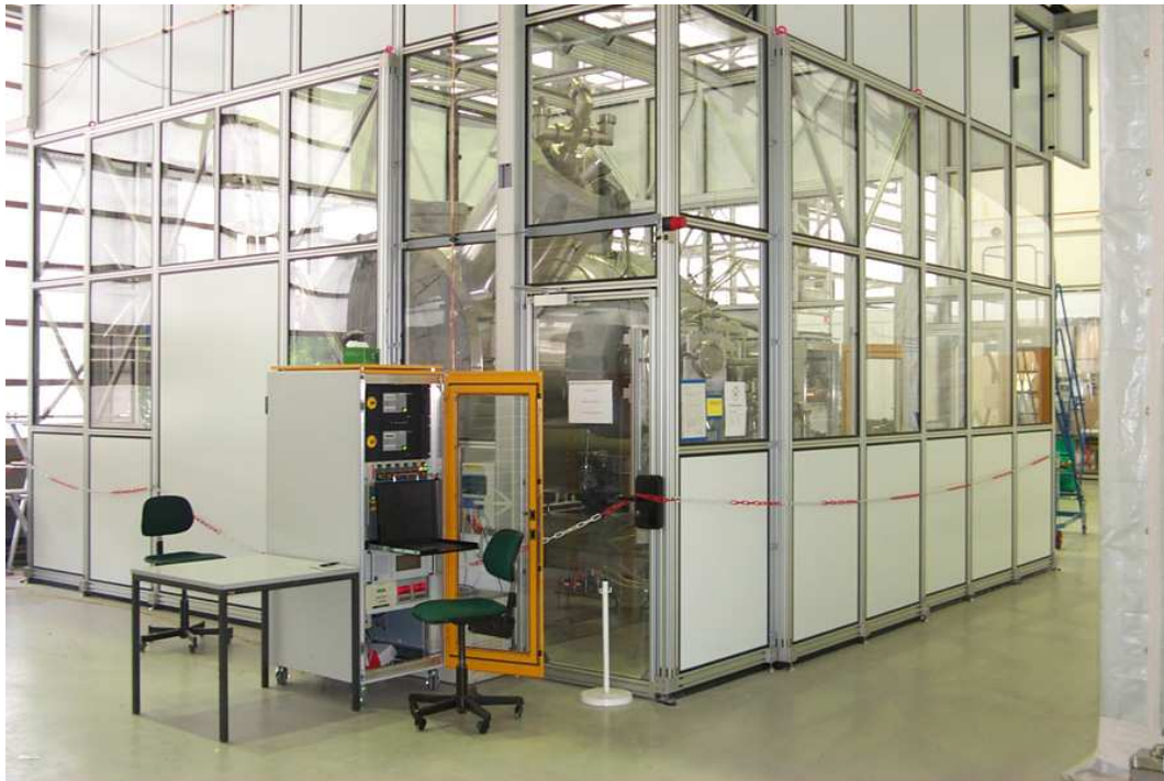
Figure 66: The dry-air compartment around the KATRIN pre-spectrometer.
