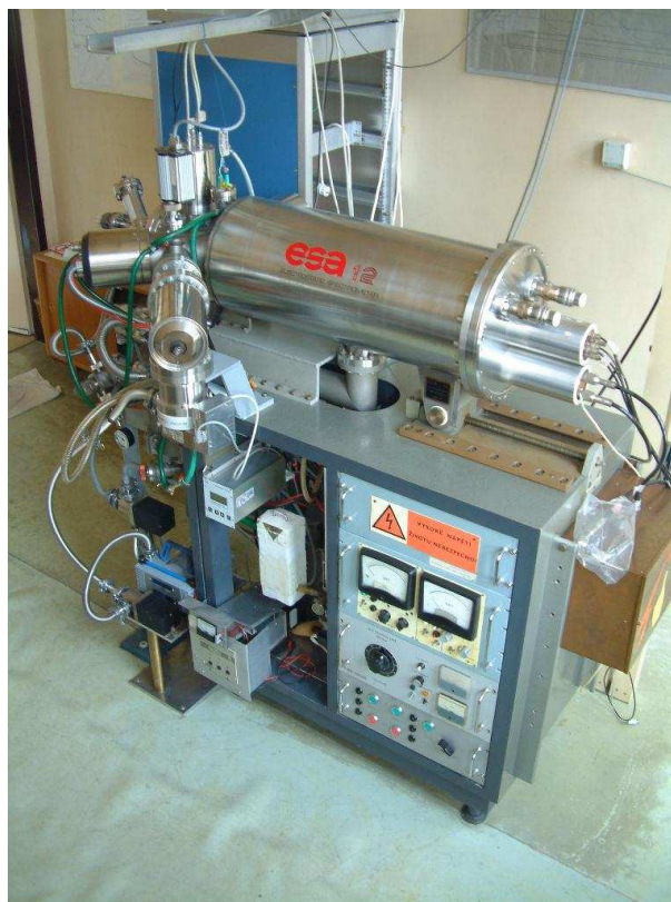
Figure 109: Electrostatic electron spectrometer ESA12 at NPI Řež. A double-pass cylindrical mirror analyzer is combined with a preacceleration/preretardation system.
