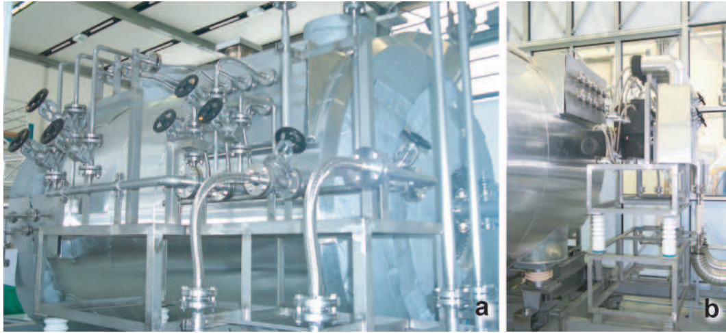
Figure 65: a: The tubes and valves distribute the oil of the heating-cooling system through different circuits of the pre-spectrometer. b: The tubes coming from the heating-cooling system are made of ceramic insulators, separating the vessel, which is on high voltage, from the rest of the system.
