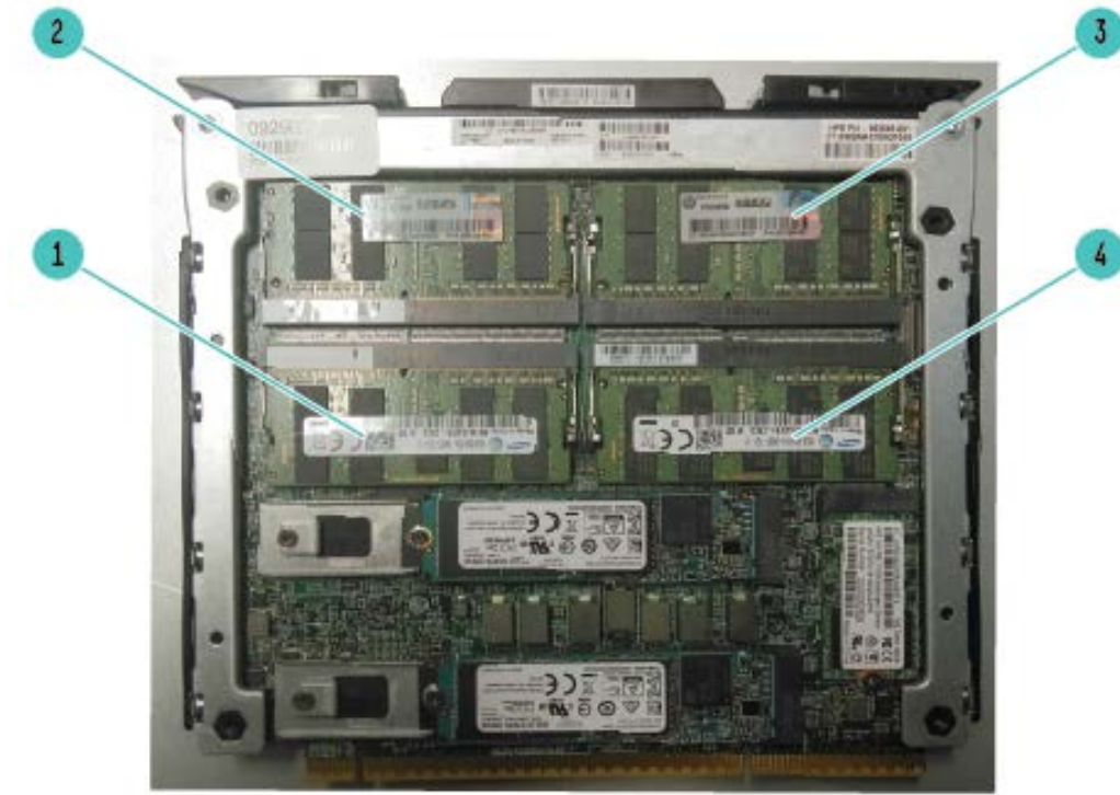
DIMM Locations on the HPE m710x/m710x-L Server
