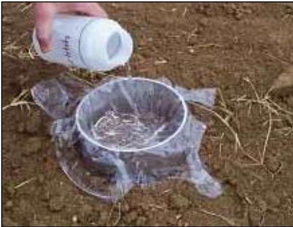
Figure 5. Illustration of use of plastic wrap to hold water in ring infiltrometer before allowing water to flow into the ring for timing of infiltration.
