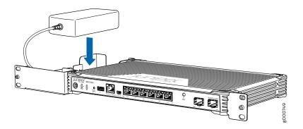
5. Lift the SRX300 and position it in the rack. Line up the bottom hole in the mounting brackets with a hole in each rack rail, making sure the SRX300 is level.
