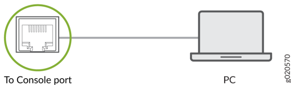
Figure 46: Connecting the MX204 Router Directly to a Management Console
