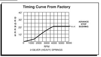
Figure 2 The Factory Equipped Curve.
