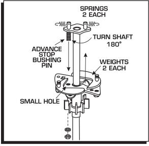
Figure 7 Locking Out the Advance.
