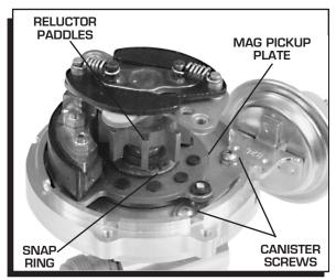
Figure 11 Removing the Vacuum Canister.
