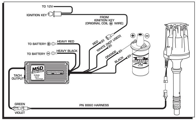
Figure 13 Wiring to an MSD 6-Series Ignition Control.
