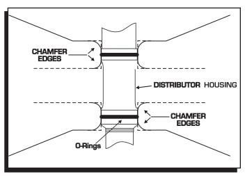
Figure 9 Modified Block for use with O-Rings.
