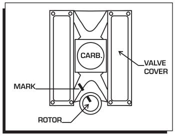
Figure 8 Marking the Rotor Location.
