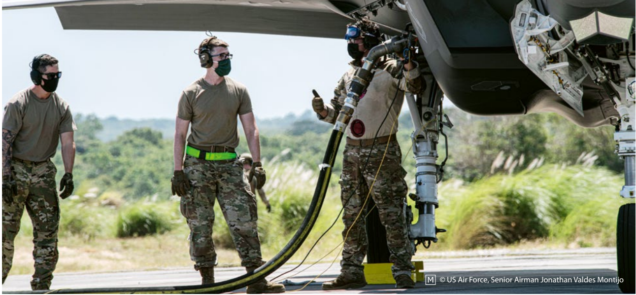
USAF Airmen perform hot-pit refuelling on an F-35A Lightning II assigned to Eielson AFB, Alaska, at Northwest Field as part of Agile Combat Employment (ACE) multi-capable Airmen training during Cope North 21 at Andersen AFB, Guam, 16 February 2021. ACE, the new warfighting concept that Pacific Air Forces is operationalizing ensures agility, deterrence, and resiliency in a contested or degraded environment.
