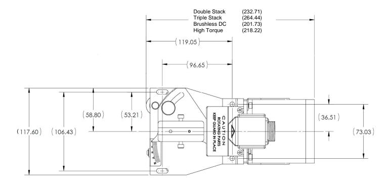
Figure 5.2 Single Ended Heavy Duty Motor/Base Module Dimensions
