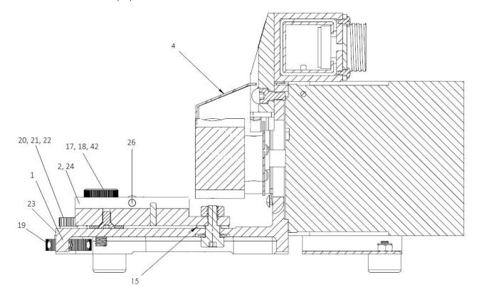
Figure 5.3 Single Ended Heavy Duty Cast Motor/Base Module
