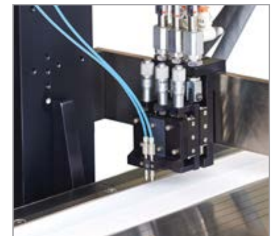
Dispensing 2 Reagent Lines onto Substrate
